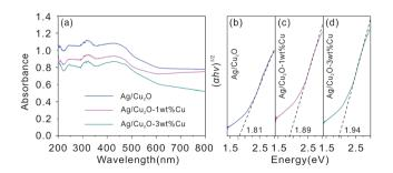
Fig. 5 (a) The UV-vis diffuses reflectance spectra for the flower-like hierarchical Ag/Cu<sub>2</sub>O composite microspheres (Sample 3), Ag/Cu<sub>2</sub>O-1 wt% Cu (Sample 1) and Ag/Cu<sub>2</sub>O-3 wt% Cu (Sample 2). (b)–(d) The corresponding  $(\alpha h \nu)^2$  versus energy  $(h \nu)$  plots of the above samples.
