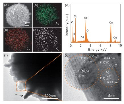
Fig. 2 SEM image (a) and EDS spectrum (e) of the flower-like hierarchical  $Ag/Cu_2O$  composite microspheres. Element mapping images of the flower-like hierarchical  $Ag/Cu_2O$  composite microspheres with "Ag" (b), "Cu" (c), and "O" (d). TEM (f) and HRTEM (g) images of the flower-like hierarchical  $Ag/Cu_2O$  composite microspheres. The black arrow in (f) marks that the nanoflake is oriented approximately perpendicular to the plane of the supporting copper TEM grid.
