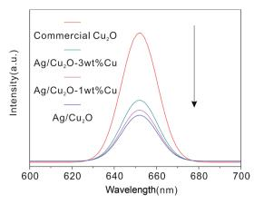
Fig. 7 PL spectra of commercial  $Cu_2O$ ,  $Ag/Cu_2O$ ,  $Ag/Cu_2O-1$  wt% Cu and  $Ag/Cu_2O-3$  wt% Cu with an excitation wavelength of 325 nm.
