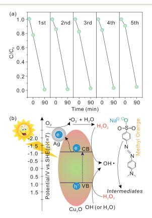
Fig. 8 (a) Photodegradation properties of the flower-like hierarchical Ag/Cu<sub>2</sub>O composite microspheres toward MO solution within five cycles under visible light illumination; (b) schematic of photo-activation of the flower-like hierarchical  $Ag/Cu_2O$  composite microspheres and degradation of MO.
