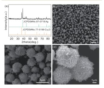
Fig. 1  $\,$  XRD pattern (a) and SEM images (b-d) of the flower-like hierarchical Ag/Cu<sub>2</sub>O composite microspheres.
