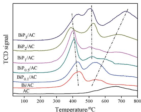
Fig. 7 H<sub>2</sub>-TPR profiles of AC, fresh Bi/AC and BiP<sub>x</sub>/AC.
