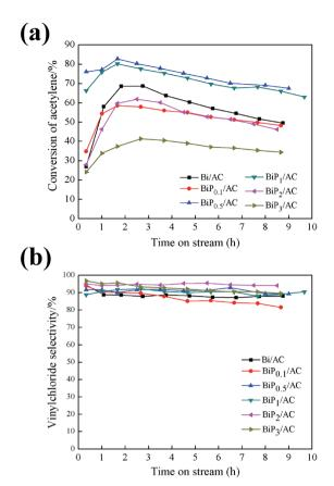
Fig. 1 Conversion of acetylene (a) and selectivity for VCM (b) over Bi/AC and BiP<sub>X</sub>/AC catalysts. Reaction conditions: temperature  $(T) = 160 \,^{\circ}$ C, GHSV =  $120 \, h^{-1}$ , and feed volume ratio  $V(HCI)/V(C_2H_2) = 1.25$ .
