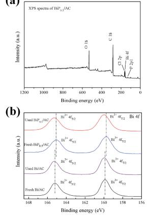
Fig. 8 (a) Wide-scan XPS spectrum of  $BiP_{0.5}/AC$ ; (b) Bi 4f XPS spectra of fresh and used Bi/AC and  $BiP_{0.5}/AC$ .
