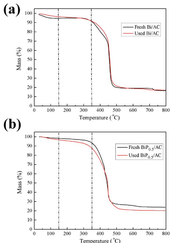
Fig. 9 TGA profiles of the fresh and used catalysts: (a) Bi/AC and (b) BiP<sub>0.5</sub>/AC.
