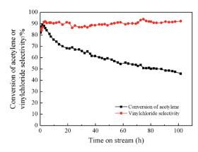
Fig. 2 Estimation of lifetime of BiP $_{0.5}$ /AC catalyst. Reaction conditions: temperature (7) = 160 °C, GHSV(C $_2$ H $_2$ ) = 30 h $^{-1}$ , and feed volume ratio  $V(HCl)/V(C_2H_2) = 1.25$ .
