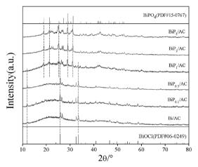
Fig. 3  $\,$  XRD patterns of fresh Bi/AC and BiP  $_{\chi}$  /AC catalysts with varying  $\rm H_3PO_4$  contents.
