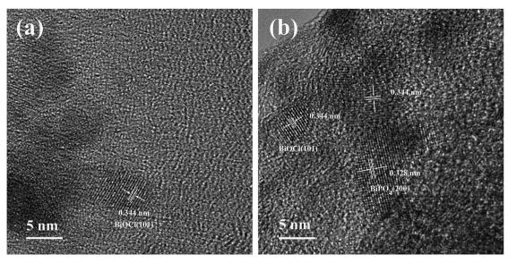
Fig. 6 HRTEM images of fresh Bi/AC (a) and BiP<sub>0.5</sub>/AC (b)
