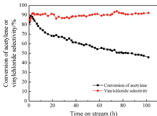
Fig. 2 Estimation of lifetime of  $\text{BiP}_{0.5}/\text{AC}$  catalyst. Reaction conditions: temperature ( $T$ ) = 160 °C,  $\text{GHSV}(\text{C}_2\text{H}_2)$  = 30  $\text{h}^{-1}$ , and feed volume ratio  $V(\text{HCl})/V(\text{C}_2\text{H}_2)$  = 1.25.
