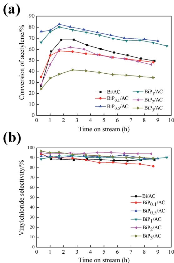
Fig. 1 Conversion of acetylene (a) and selectivity for VCM (b) over Bi/AC and BiP<sub>x</sub>/AC catalysts. Reaction conditions: temperature ( $T$ ) = 160 °C, GHSV = 120 h<sup>-1</sup>, and feed volume ratio  $V(\text{HCl})/V(\text{C}_2\text{H}_2) = 1.25$ .
