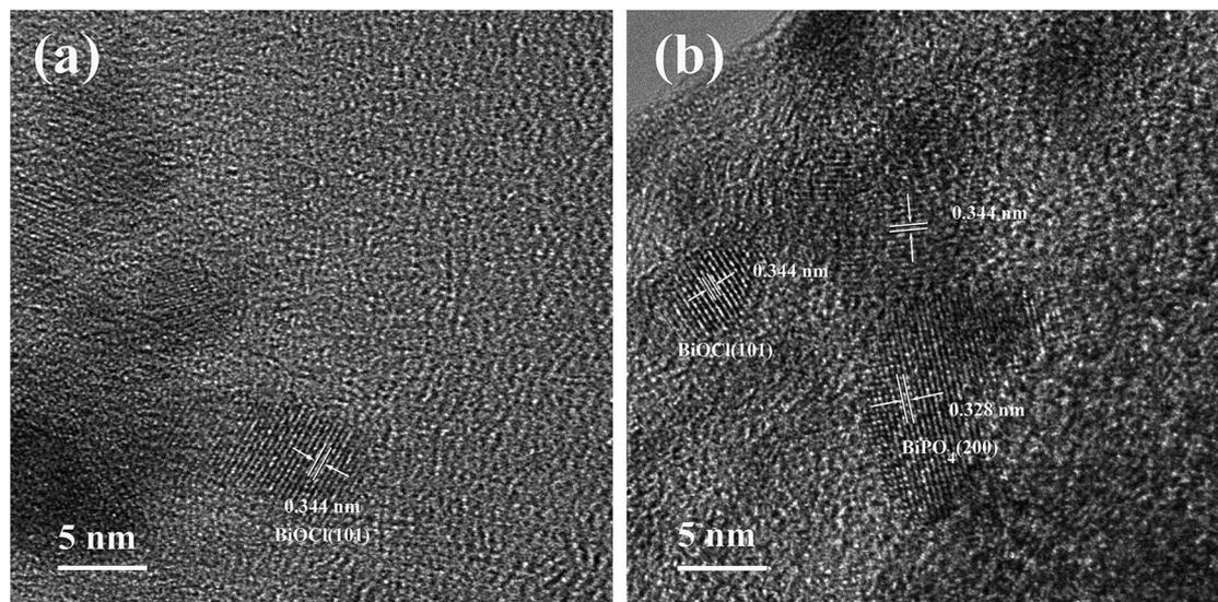
Fig. 6 HRTEM images of fresh Bi/AC (a) and BiP<sub>0.5</sub>/AC (b).
