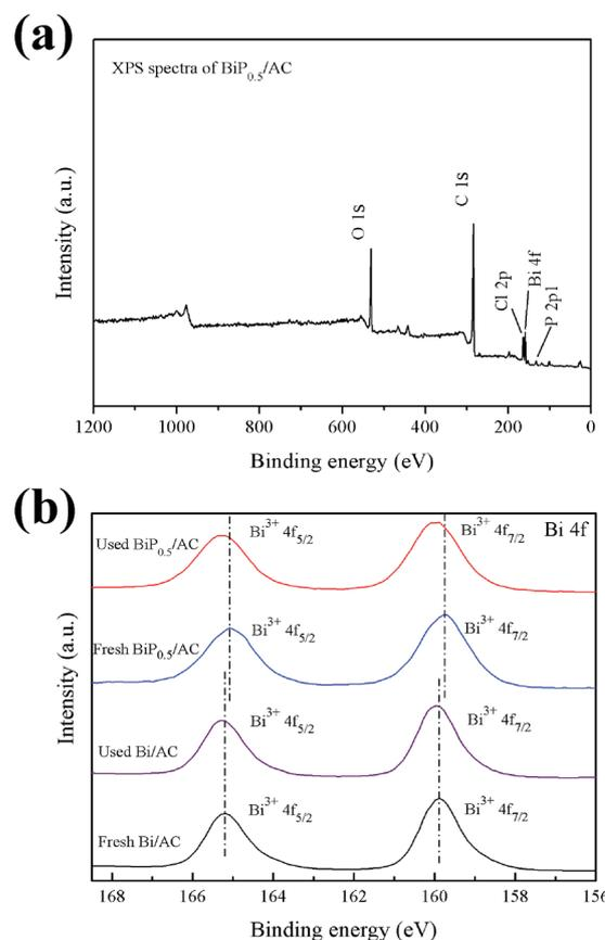
Fig. 8 (a) Wide-scan XPS spectrum of BiP<sub>0.5</sub>/AC; (b) Bi 4f XPS spectra of fresh and used Bi/AC and BiP<sub>0.5</sub>/AC.
