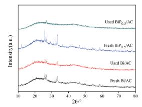
Fig. 4 XRD patterns of fresh and used Bi/AC and BiP<sub>0.5</sub>/AC catalysts.
