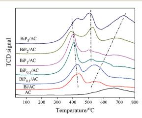
Fig. 7  $H_2$ -TPR profiles of AC, fresh Bi/AC and BiP<sub>X</sub>/AC.
