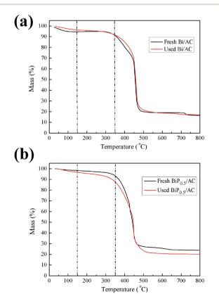
Fig. 9 TGA profiles of the fresh and used catalysts: (a) Bi/AC and (b) BiP<sub>0.5</sub>/AC.
