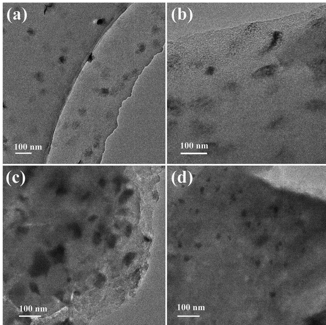
Fig. 5 TEM images of Bi/AC (a and c) and BiP<sub>0.5</sub>/AC (b and d) before (a and b) and after (c and d) the reaction.
