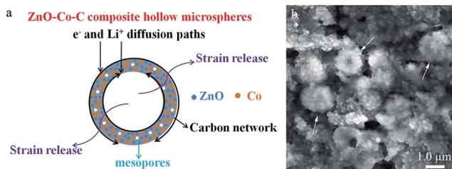
Fig. 7 (a) Schematic of the structural merits of ZnO-Co-C composite hollow microspheres. (b) SEM micrograph of ZnO-Co-C composite hollow microspheres after 100 cycles.
