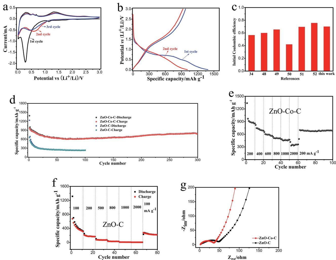
**Fig. 6** (a) The CV profiles, (b) galvanostatic potential–capacity curves of ZnO–Co–C. (c) The comparison of initial coulombic efficiency of ZnO-based electrodes. (d) The cycling performances for ZnO–Co–C composites at  $200 \text{ mA g}^{-1}$  and ZnO–C solid microspheres at  $100 \text{ mA g}^{-1}$ . The rate performances at varied current density of (e) ZnO–Co–C hollow composites and (f) ZnO–C solid microspheres. (g) The electrochemical impedance spectra of ZnO–Co–C and ZnO–C composites.
