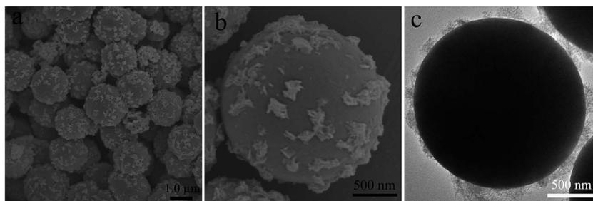
Fig. 1 The (a and b) SEM and (c) TEM micrographs of zinc citrate solid microspheres with rough surfaces.
