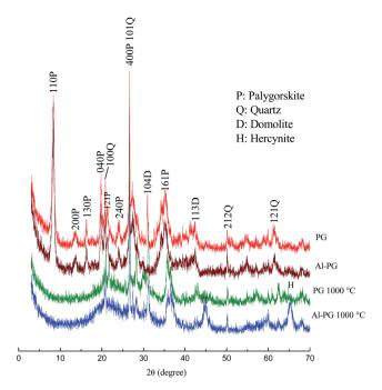
Fig. 1 XRD patterns of Al-PG, PG and their calcinates
