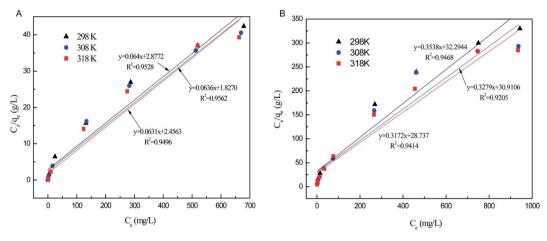
Fig. 6 The Langmuir isotherm plots of phosphate adsorption on Al-PG (A) and PG (B) (pH = 5, t = 24 h, T = 298 K).
