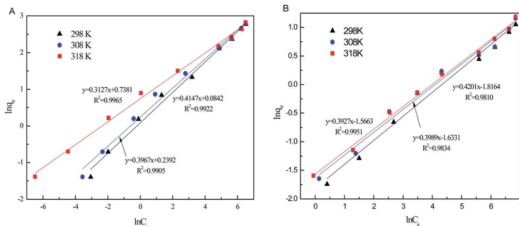
Fig. 7 The Freundlich isotherm plots of phosphate adsorption on Al-PG (A) and PG (B) ( $\text{pH} = 5$ ,  $t = 24 \text{ h}$ ,  $T = 298 \text{ K}$ ).
