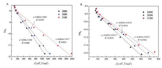
Fig. 8 The D-R isotherm plots of phosphate adsorption on Al-PG (A) and PG (B) (pH = 5, t = 24 h, T = 298 K).
