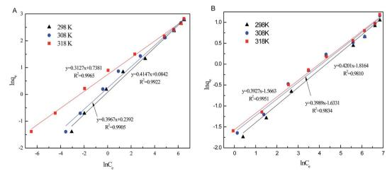
The Freundlich isotherm plots of phosphate adsorption on Al-PG (A) and PG (B) (pH = 5, t = 24 h, T = 298 K).
