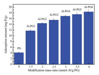
Fig. 3 Effect of modification mass ratio on adsorption capacity ( $C_0 = 1000 \text{ mg L}^{-1}$ , pH = 5, t = 24 h, T = 298 K).
