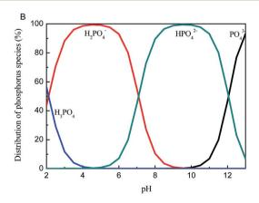
Fig. 4 (A) Effect of initial pH on phosphate adsorption on Al-PG and PG; (B) distribution of phosphorus species in aqueous solutions ( $C_0 = 500 \text{ mg L}^{-1}$ , t = 24 h, T = 298 K).
