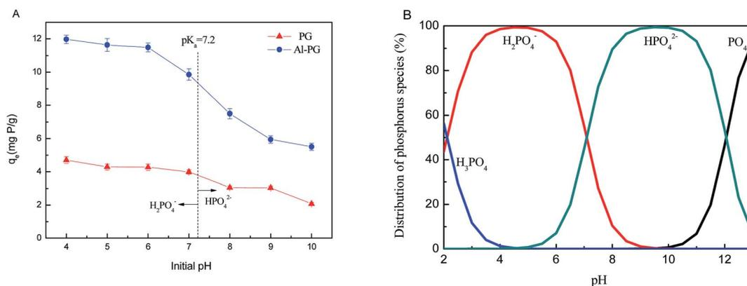
Fig. 4 (A) Effect of initial pH on phosphate adsorption on Al-PG and PG; (B) distribution of phosphorus species in aqueous solutions ( $C_0 = 500 \text{ mg L}^{-1}$ ,  $t = 24 \text{ h}$ ,  $T = 298 \text{ K}$ ).
