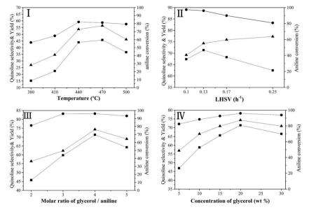
Fig. 6 Effect of temperature (I), LHSV of aniline (II), molar ratio of glycerol/aniline (III) and concentration of glycerol (IV) over the Ni/H $\beta$ -At catalyst. aniline conversion (- $\bullet$ -), quinoline selectivity (- $\Delta$ -) and quinoline yield (- $\blacksquare$ -).
