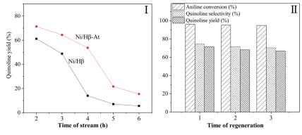
Fig. 7 The stability of the Ni/H $\beta$  and Ni/H $\beta$ -At catalysts (I) and regenerability of Ni/H $\beta$ -At (II). Reaction condition: catalyst weight = 1.0 g; temperature = 470 °C; LHSV (aniline) = 0.13 h<sup>-1</sup>; molar ratio of aniline/glycerol = 1/4; concentration of glycerol agueous solution = 20 wt%.
