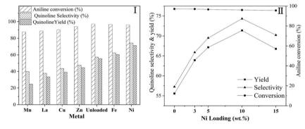
Fig. 5 Effect of the different metal (I) and loading amount of Ni (II) supported on H $\beta$ -At. Reaction condition: catalyst weight = 1.0 g; temperature = 470 °C; molar ratio of aniline/glycerol = 1/4; LHSV (aniline) = 0.13 h<sup>-1</sup>; concentration of glycerol aqueous solution = 20 wt%.
