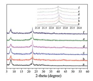
Fig. 1 XRD patterns for the fresh and deactivated catalysts. (a) H $\beta$ ; (b) Ni/H $\beta$ ; (c) deactivated Ni/H $\beta$ ; (d) H $\beta$ -At; (e) Ni/H $\beta$ -At; (f) deactivated H $\beta$ -At. (The inset shows the enlargement of the predominant peaks in the XRD patterns.)
