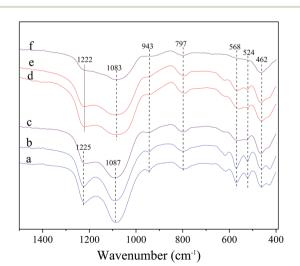
Fig. 2 FT-IR spectra of the fresh and deactivated catalysts. (a) Hβ; (b) Ni/Hβ; (c) deactivated Ni/Hβ; (d) Hβ-At; (e) Ni/Hβ-At; (f) deactivated Hβ-At.
