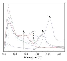
Fig. 4  $NH_3$ -TPD profiles for the fresh and deactivated catalysts. (a)  $H\beta$ ; (b)  $H\beta$ -At; (c)  $Ni/H\beta$ ; (d)  $Ni/H\beta$ -At; (e) deactivated  $Ni/H\beta$ -At; (f) regenerated  $Ni/H\beta$ -At.
