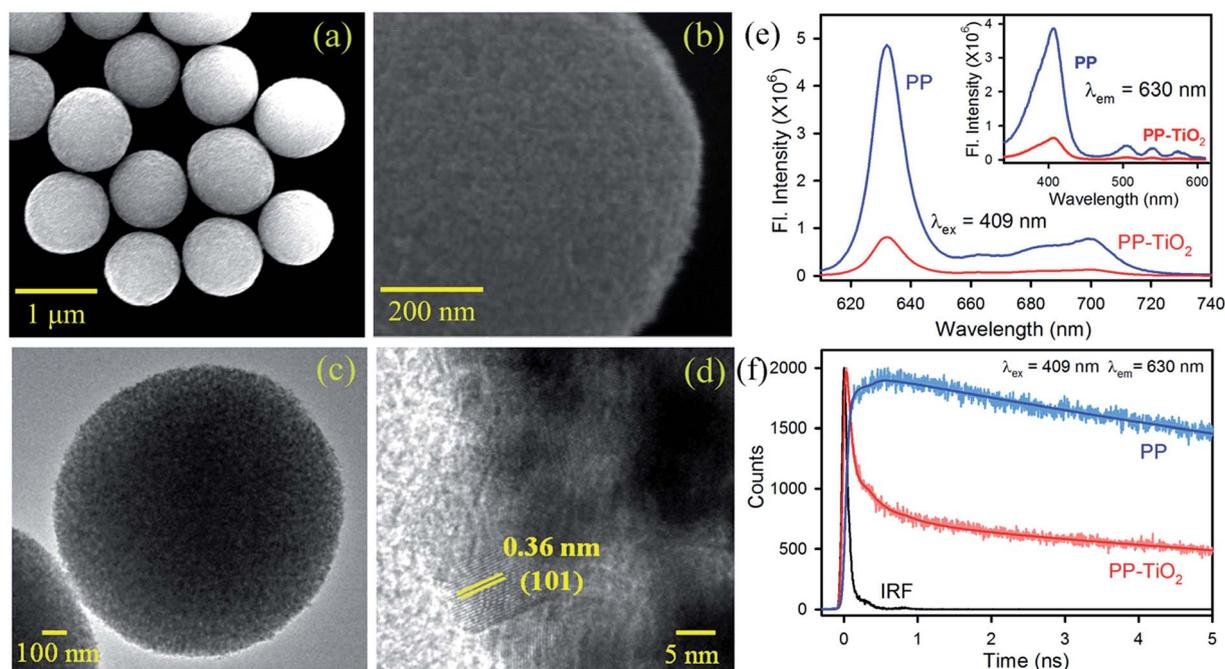
**Fig. 1** (a and b) SEM and (c and d) TEM images of the TiO<sub>2</sub> MS. (e) Room-temperature PL spectra (excitation at 409 nm) of free PP (blue) and PP-TiO<sub>2</sub> MS (red). The inset shows the excitation spectra monitored at 630 nm. (f) Fluorescence decay profiles of PP (blue) and PP-TiO<sub>2</sub> MS (red) at 630 nm (with excitation at 409 nm).
