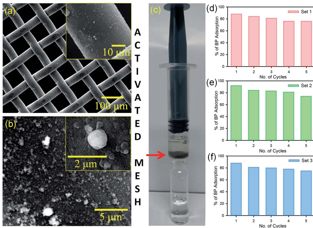
Fig. 3 (a and b) SEM images of the PP-sensitized TiO<sub>2</sub> MS on stainless steel mesh (activated mesh). (c) The prototype flow device fabricated using the activated mesh. (d–f) BP removal using the flow device in different sets. Chemical recharging of the activated mesh using acetonitrile was performed after each set.
