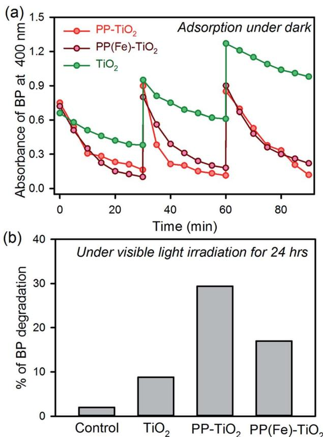
**Fig. 2** (a) The adsorption kinetics of BP dispersed in water in the presence of TiO<sub>2</sub> MS, PP-TiO<sub>2</sub> MS, and PP(Fe)-TiO<sub>2</sub> MS under dark conditions. (b) The degradation of BP adsorbed on the surface of different materials under visible light irradiation for 24 h.
