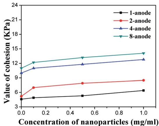
Fig. 8 Increment of the cohesion of soil near the anode due to electroosmosis and NPs injection.
