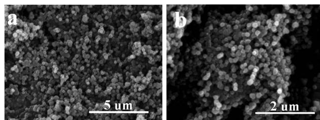
Fig. 3 SEM images of  $\text{SiO}_2$  NPs (a) and  $\text{SiO}_2@/\text{Al}_2\text{O}_3$  core-shell NPs (b).
