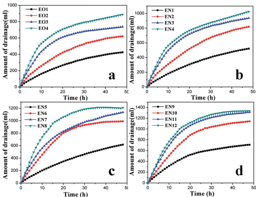
Fig. 7 Evolution of drained water volume with time during treatment with electroosmosis and injection of positively charged NPs: (a)  $0 \text{ mg ml}^{-1}$ ; (b)  $0.1 \text{ mg ml}^{-1}$ ; (c)  $0.5 \text{ mg ml}^{-1}$ ; (d)  $1.0 \text{ mg ml}^{-1}$ . Replicate experiments suggested variabilities within  $\pm 7\%$ .
