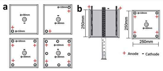
Fig. 1 Schematic configuration of electroosmotic cells (a) top view (b) profile.
