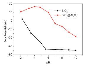
Fig. 2 Zeta potential of  $SiO_2$  NPs vs.  $SiO_2@Al_2O_3$  core—shell NPs as a function of pH.
