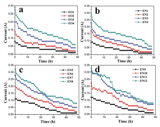
Fig. 5 Evolution of electric current with time during treatment with electroosmosis and injection of positively charged NPs: (a) 0 mg ml<sup>-1</sup>; (b) 0.1 mg ml<sup>-1</sup>; (c) 0.5 mg ml<sup>-1</sup>; (d) 1.0 mg ml<sup>-1</sup>. Replicate experiments suggested variabilities within  $\pm 8\%$ .
