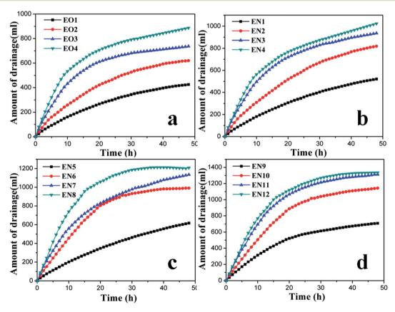
Fig. 7 Evolution of drained water volume with time during treatment with electroosmosis and injection of positively charged NPs: (a) 0 mg ml $^{-1}$ ; (b) 0.1 mg ml $^{-1}$ ; (c) 0.5 mg ml $^{-1}$ ; (d) 1.0 mg ml $^{-1}$ . Replicate experiments suggested variabilities within  $\pm 7\%$ .
