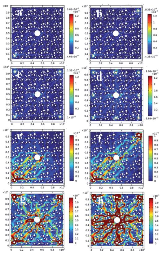
Fig. 12 Variation of electroosmotic coefficient of electroosmosis process without (a-d) and with 1 mg ml<sup>-1</sup> NPs (e-h).
