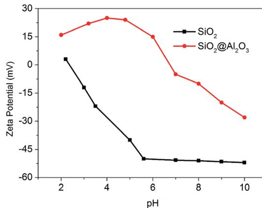
Fig. 2 Zeta potential of  $\text{SiO}_2$  NPs vs.  $\text{SiO}_2@/\text{Al}_2\text{O}_3$  core-shell NPs as a function of pH.
