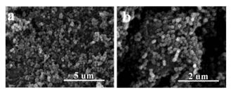
Fig. 3 SEM images of SiO<sub>2</sub> NPs (a) and SiO<sub>2</sub>@Al<sub>2</sub>O<sub>3</sub> core-shell NPs (b).
