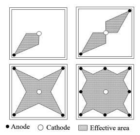
Fig. 6 Schematic illustrating the effect of anode configuration on the distribution of effective area during electroosmosis.<sup>19</sup>
