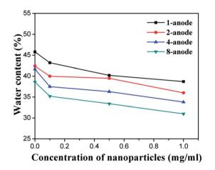
Fig. 10 The water content of the treated soil near the anode, as a function of concentration of NPs.
