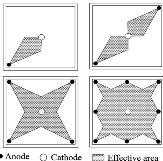
Fig. 6 Schematic illustrating the effect of anode configuration on the distribution of effective area during electroosmosis.<sup>19</sup>
