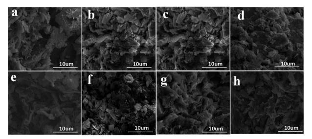
Fig. 11 Representative SEM micrographs of the soil near cathode after electroosmosis only or with injection of positively charged NPs: (a) EO1 (b) EO2 (c) EO3 (d) EO4 (e) EN9 (f) EN10 (g) EN11 (h) EN12.
