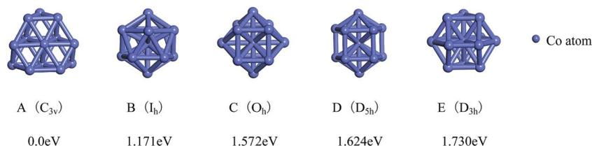
Fig. 1 The referenced total binding energies (see text for details) and symmetries of the ground-state geometry and the four high-symmetric configurations of Co<sub>13</sub>.
