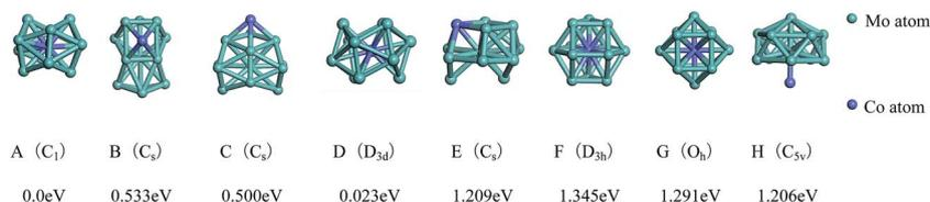
Fig. 4 The referenced total binding energies (see text for details) and symmetries of the ground-state geometry, the low-lying isomers and the four high-symmetric configurations of  $Mo_{12}Co$ .
