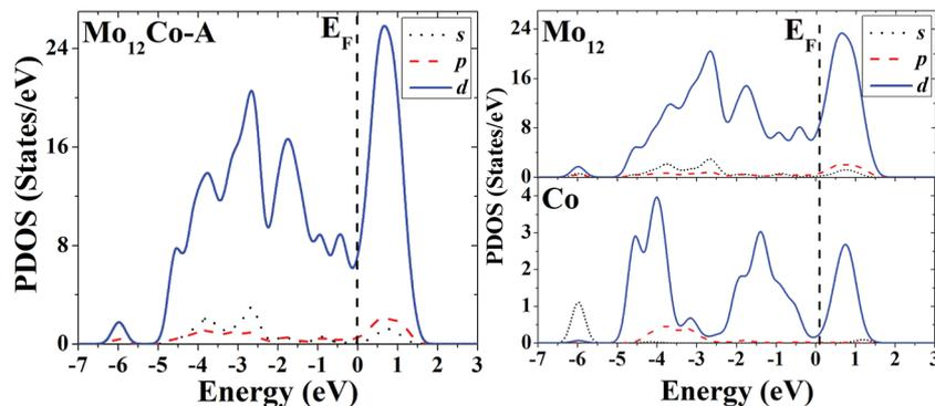
Fig. 13 Partial density of states (PDOS) of the whole (left) and components (right) of the ground-state geometry of  $\text{Mo}_{12}\text{Co}$ .
