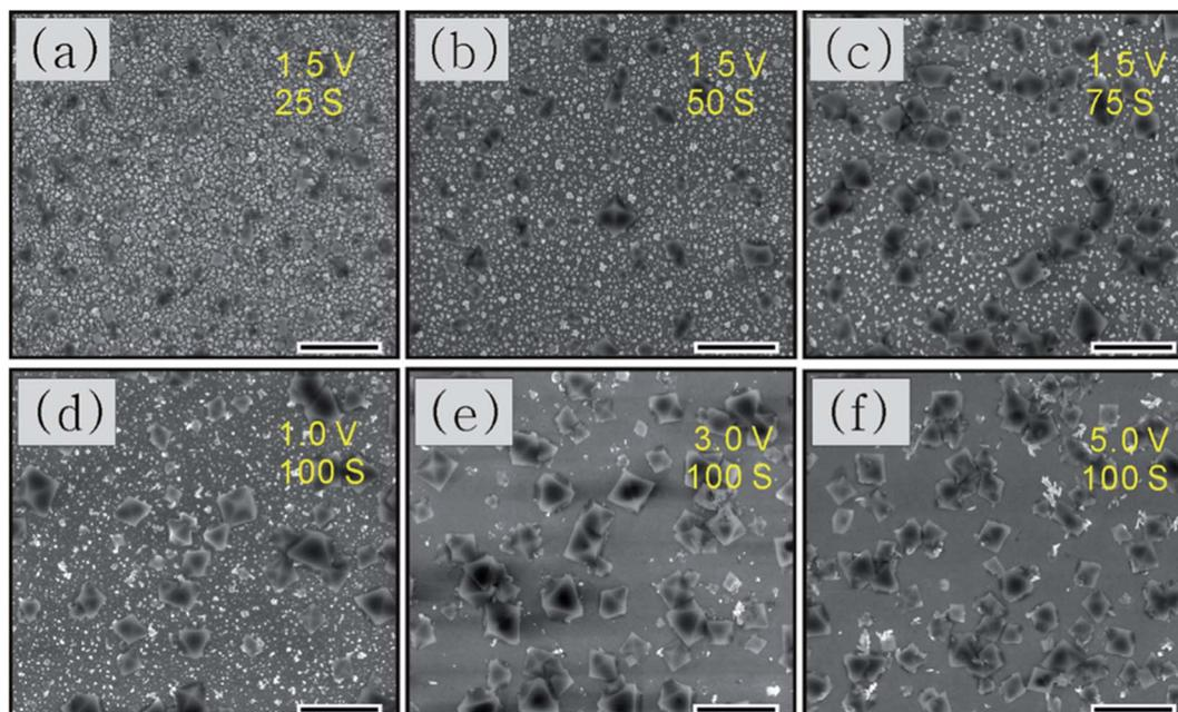
Fig. 4 SEM images of HKUST-1/ITO, formed by electro-oxidation of Cu/ITO in a solvent ( $v_{\text{EtOH}}/v_{\text{H}_2\text{O}} = 3 : 1$ ) containing 25 mmol L<sup>-1</sup> BTC as a linking agent and 50 mmol L<sup>-1</sup> TBAP as a supporting electrolyte at 1.5 V for (a) 25 s, (b) 50 s, or (c) 75 s, and at different potentials of (d) 1.0 V, (e) 3.0 V, or (f) 5.0 V for 100 s. The scale bar is 2  $\mu\text{m}$  long.
