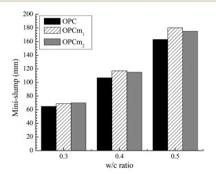
Fig. 4 Influence of the admixed micelles on the mini-slump flow of cement paste.
