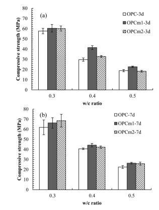
Fig. 7 Compressive strength of cement pastes with different w/c ratios: (a) 3 days and (b) 7 days.
