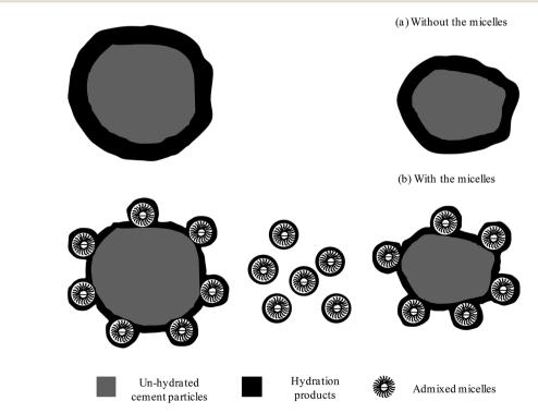
A hypothesis on the acceleration of cement hydration by the admixed micelles.
