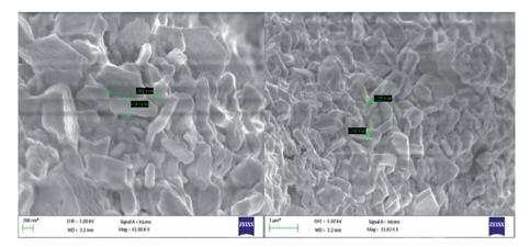
Fig. 5 FESEM morphology of the sample (Bi<sub>2</sub>Te<sub>3</sub>)<sub>25</sub>(CdTe)<sub>75</sub> having nanorods approximately 240 nm in size.
