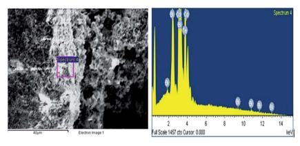
Fig. 6 EDX spectrum of (Bi<sub>2</sub>Te<sub>3</sub>)<sub>25</sub>(CdTe)<sub>75</sub> sample.
