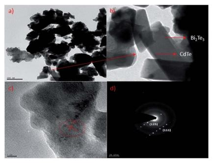
Fig. 3 (a) & (b) Core/shell nanostructure of  $(Bi_2Te_3)_{25}(CdTe)_{75}$ ; (c) & (d) electron diffraction (SAED) shows the crystalline structure of  $Bi_2Te_3/CdTe$  in sample  $(Bi_2Te_3)_{25}(CdTe)_{75}$ .
