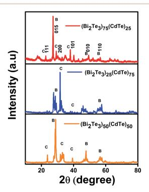
Fig. 2  $\,$  XRD patterns of Bi<sub>2</sub>Te<sub>3</sub>/CdTe powder composites. XRD data for comparison of bismuth telluride percentage in cadmium telluride.
