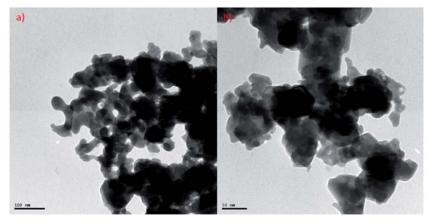
Fig. 4 TEM images of powder samples of (a) (Bi<sub>2</sub>Te<sub>3</sub>)<sub>75</sub>(CdTe)<sub>25</sub> and (b) (Bi<sub>2</sub>Te<sub>3</sub>)<sub>50</sub>(CdTe)<sub>50</sub>.
