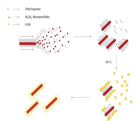
Fig. 1 Self-assembly of Bi<sub>2</sub>Te<sub>3</sub>/CdTe with the help of a PVA polymer.
