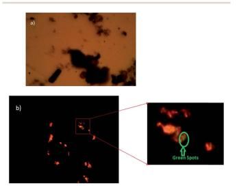
Fig. 7 (a) Transmittance image of  $Bi_2Te_3/CdTe$  nanorods and (b) the reflectance image of  $Bi_2Te_3/CdTe$  nanorods.
