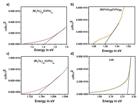
Fig. 8 The energy band gap graph of samples (a)  $(Bi_2Te_3)_{25}(CdTe)_{75}$ , (b)  $(Bi_2Te_3)_{75}(CdTe)_{25}$ , (c)  $(Bi_2Te_3)_{50}(CdTe)_{50}$ , and (d) CdS layer in the fabricated device.
