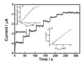
Fig. 6 Amperometric responses of CS/[GOx]<sub>5</sub>/[CNCs]<sub>5</sub>/GCE at an operating potential of -400 mV with successive additions of 0.1 M glucose in PBS (0.1 M, pH 7.2). Inset (a): plot of catalytic current of the modified electrode vs. glucose concentration. Inset (b): Lineweaver-Burk plot for  $K_{\rm m}^{\rm app}$  determination.
