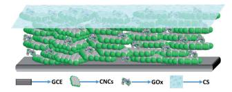
Fig. 1 Schematic structure of CS/GOx/CNCs/GCE.
