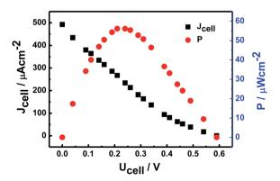
Fig. 7 Typical power density vs. cell voltage and current density vs. cell voltage curves of CS/[GOx]<sub>5</sub>/[CNCs]<sub>5</sub>/GCE in air-saturated PBS (pH 7.2) containing 10 mM glucose against Pt electrode as cathode.
