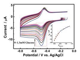
Fig. 4 CV curves of  $CS/[GOx]_5/[CNCs]_5/GCE$  in air-saturated PBS (0.1 M, pH 7.2) solution with various concentrations of glucose. Scan rate: 100 m s<sup>-1</sup>. Inset: calibration curve of the linear dependence of cathodic peak current on the glucose concentration.
