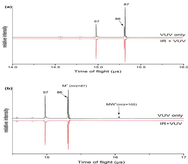
**Fig. 1** (a) Mass spectra of morpholine cation and fragment ions which are generated in the 118 nm light with the IR light on/off. (b) Mass spectrum of morpholine monohydrated clusters and fragment ions which are generated in the 118 nm light with the IR light on/off. Both mass spectrums were observed with a time of flight mass spectrometer.
