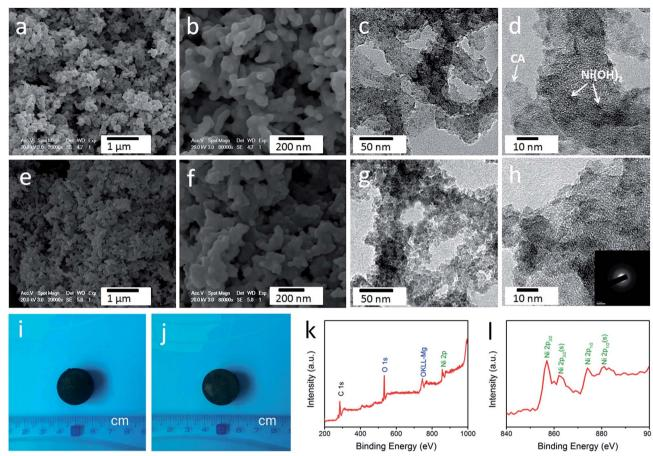
Fig. 3 (a and b) SEM images and (c and d) TEM images of  $CA/Ni(OH)_2/0.30$ . (e and f) SEM images and (g and h) TEM images of  $CA/Ni(OH)_2/0.75$ . Photographs of (i)  $CA/Ni(OH)_2/0.30$  and (j)  $CA/Ni(OH)_2/0.75$ . (k) XPS spectra and (l) Ni 2p XPS spectra of  $CA/Ni(OH)_2/0.75$ . The inset is the selected area electron diffraction pattern of  $CA/Ni(OH)_2/0.75$ .
