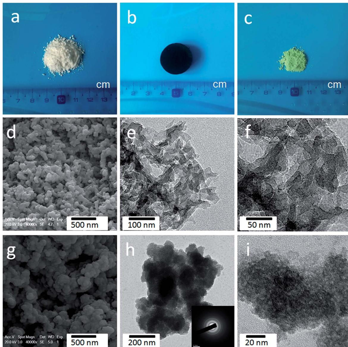
Fig. 2 Photographs of (a) microcrystalline cellulose powder, (b) cellulose-derived CA, and (c)  $\text{Ni}(\text{OH})_2$ . (d) SEM images and (e and f) TEM images of cellulose-derived CA. (g) SEM images and (h and i) TEM images of  $\text{Ni}(\text{OH})_2$ .
