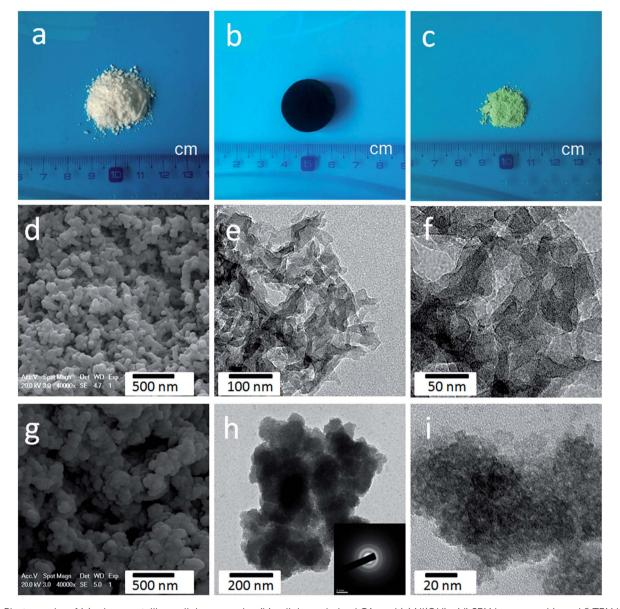
Fig. 2 Photographs of (a) microcrystalline cellulose powder, (b) cellulose-derived CA, and (c)  $Ni(OH)_2$ . (d) SEM images and (e and f) TEM images of cellulose-derived CA. (g) SEM images and (h and i) TEM images of  $Ni(OH)_2$ .
