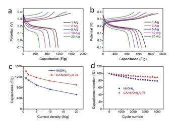
Fig. 6 Galvanostatic charge/discharge curves of (a) Ni(OH)<sub>2</sub> and (b) CA/Ni(OH)<sub>2</sub>/0.75 at different constant current densities, ranging from 1 to 20 A g $^{-1}$ . (c) Specific capacitances at various discharge current densities. Here, the capacitances of CA/Ni(OH)<sub>2</sub>/0.75 are based on the mass of the entire CA/Ni(OH)<sub>2</sub> electrodes. (d) Cycling performance measured at a current density of 20 A g $^{-1}$  in a potential range of -0.1 to 0.4 V.
