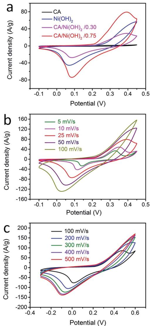
Fig. 5 (a) CV curves of cellulose-derived CA, Ni(OH)<sub>2</sub>, and CA/Ni(OH)<sub>2</sub> composite at a scan rate of 25 mV s<sup>-1</sup>. (b) CV curves of CA/Ni(OH)<sub>2</sub>/0.75 at different scan rates ranging from 5 to 100 mV s<sup>-1</sup>. (c) CV curves of CA/Ni(OH)<sub>2</sub>/0.75 in a potential window of -0.3 to 0.6 V at scan rates of 100, 200, 300, 400 and 500 mV s<sup>-1</sup>.
