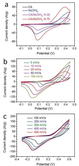
Fig. 5 (a) CV curves of cellulose-derived CA, Ni(OH) $_2$ , and CA/Ni(OH) $_2$  composite at a scan rate of 25 mV s $^{-1}$ . (b) CV curves of CA/Ni(OH) $_2$ / 0.75 at different scan rates ranging from 5 to 100 mV s $^{-1}$ . (c) CV curves of CA/Ni(OH) $_2$ /0.75 in a potential window of -0.3 to 0.6 V at scan rates of 100, 200, 300, 400 and 500 mV s $^{-1}$ .
