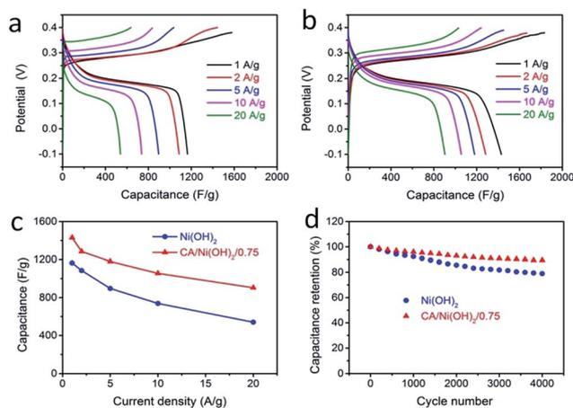
Fig. 6 Galvanostatic charge/discharge curves of (a) Ni(OH)<sub>2</sub> and (b) CA/Ni(OH)<sub>2</sub>/0.75 at different constant current densities, ranging from 1 to 20 A g<sup>-1</sup>. (c) Specific capacitances at various discharge current densities. Here, the capacitances of CA/Ni(OH)<sub>2</sub>/0.75 are based on the mass of the entire CA/Ni(OH)<sub>2</sub> electrodes. (d) Cycling performance measured at a current density of 20 A g<sup>-1</sup> in a potential range of -0.1 to 0.4 V.
