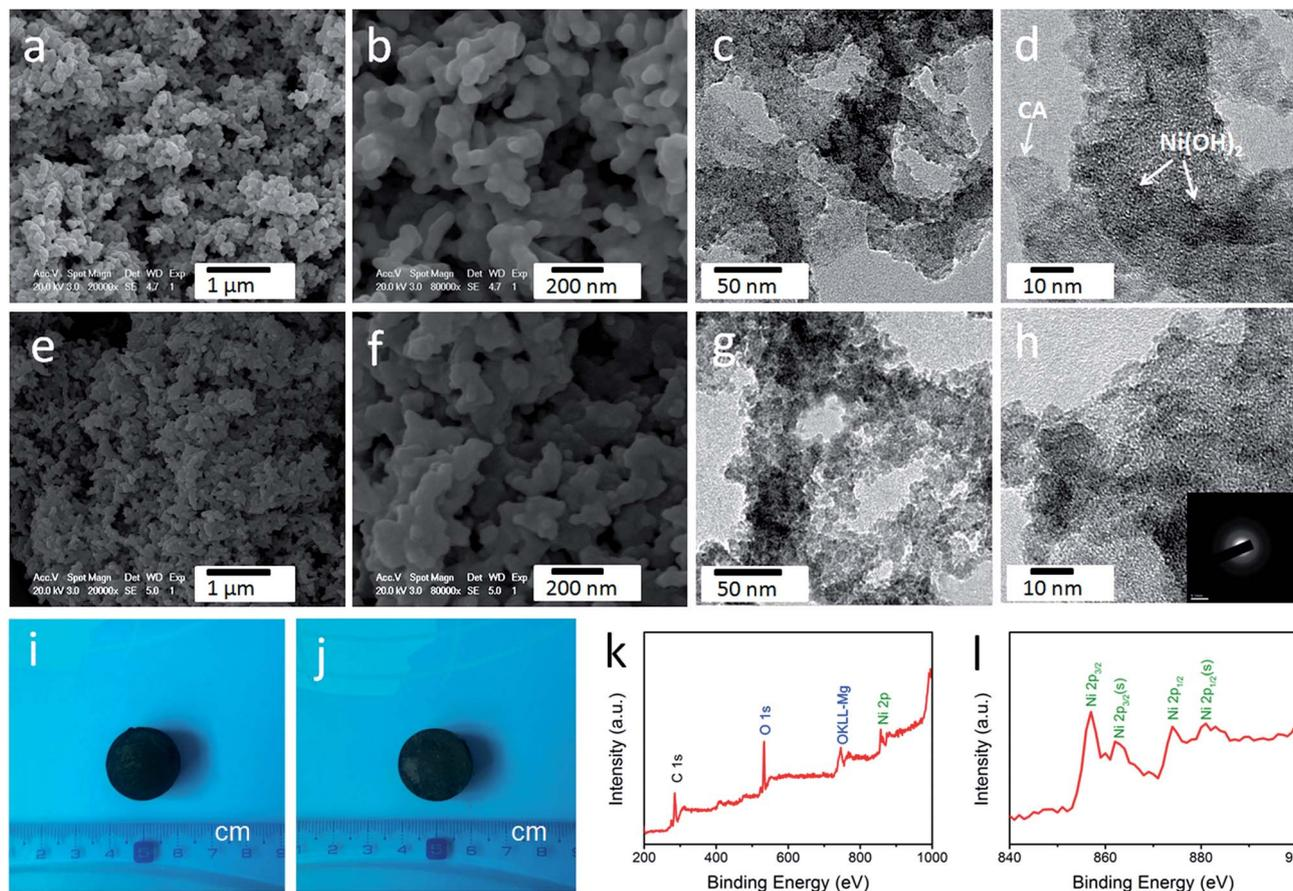
Fig. 3 (a and b) SEM images and (c and d) TEM images of CA/Ni(OH)<sub>2</sub>/0.30. (e and f) SEM images and (g and h) TEM images of CA/Ni(OH)<sub>2</sub>/0.75. Photographs of (i) CA/Ni(OH)<sub>2</sub>/0.30 and (j) CA/Ni(OH)<sub>2</sub>/0.75. (k) XPS spectra and (l) Ni 2p XPS spectra of CA/Ni(OH)<sub>2</sub>/0.75. The inset is the selected area electron diffraction pattern of CA/Ni(OH)<sub>2</sub>/0.75.
