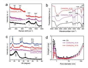
Fig. 4 (a) Raman spectra and (b) FTIR spectra of the cellulose-derived CA and CA/Ni(OH)<sub>2</sub> composite. (c) XRD patterns of cellulose-derived CA, Ni(OH)<sub>2</sub>, and CA/Ni(OH)<sub>2</sub> composite. (d) Pore size distributions of cellulose-derived CA and CA/Ni(OH)<sub>2</sub> composite.
