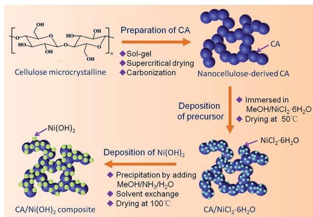
Fig. 1 Schematic of the fabrication process of the cellulose-derived CA/Ni(OH)<sub>2</sub> composite.
