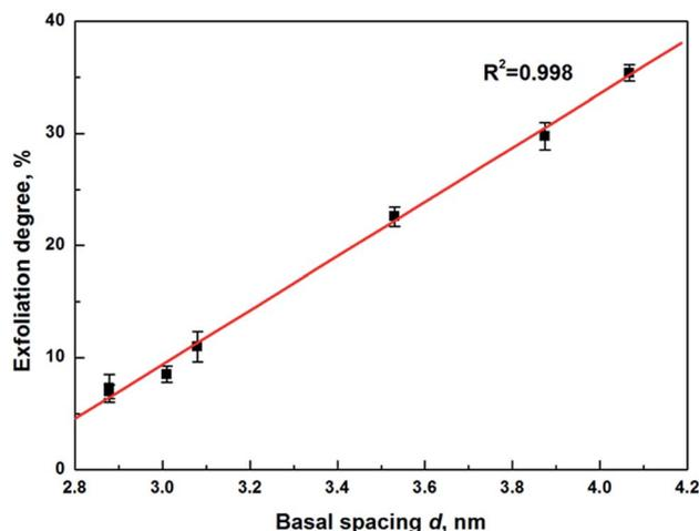
Fig. 4 Exfoliation degree of muscovite as a function of basal spacing (error bars: one standard deviation).
