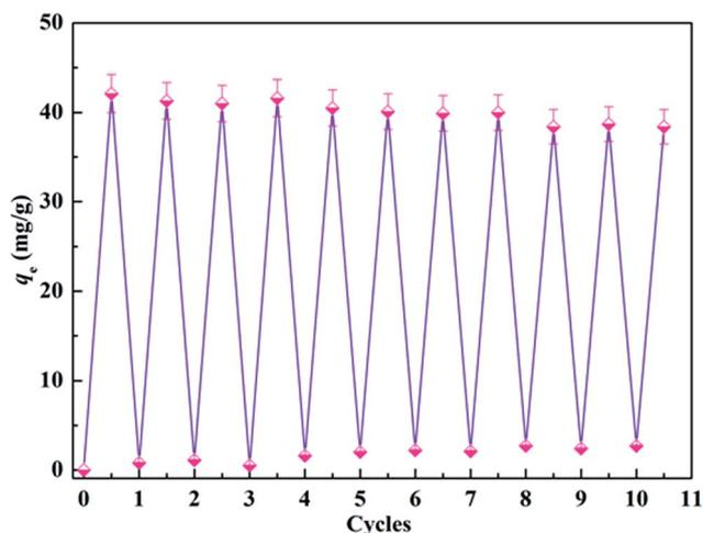
Fig. 8 Change in the adsorption capacity of CA-CS/HHF materials upon increasing the cycle number up to 10.
