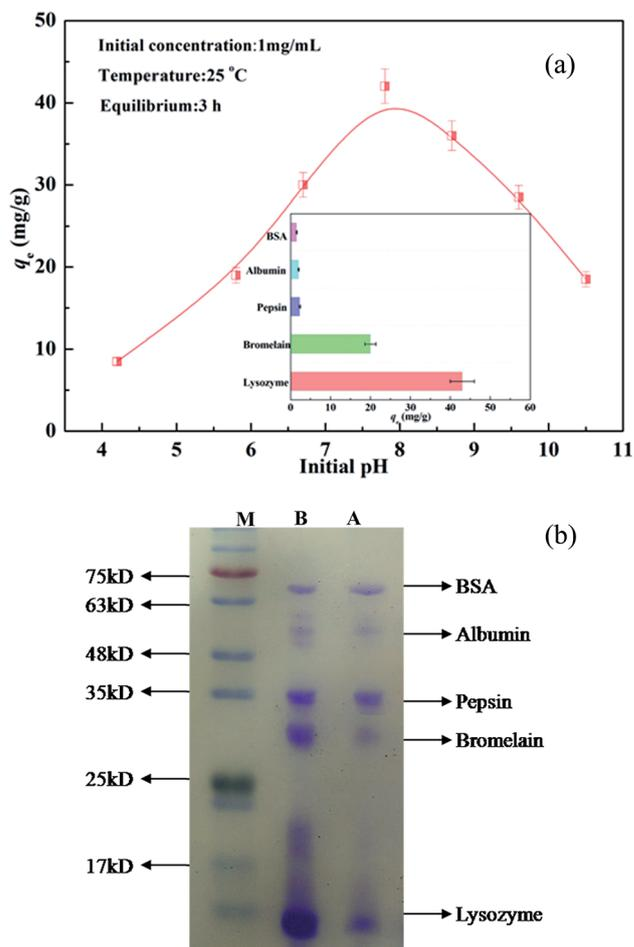
Fig. 5 (a) The observed adsorption of LYZ ( $1 \text{ mg mL}^{-1}$ ) onto CA-CS/HHF composite beads. Inset image: adsorption capacities toward different types of separate proteins. (b) SDS-PAGE analysis of the purification of a protein mixture: M, protein marker; lanes B and A, protein mixture before and after adsorption on CA-CS/HHF hybrid beads.
