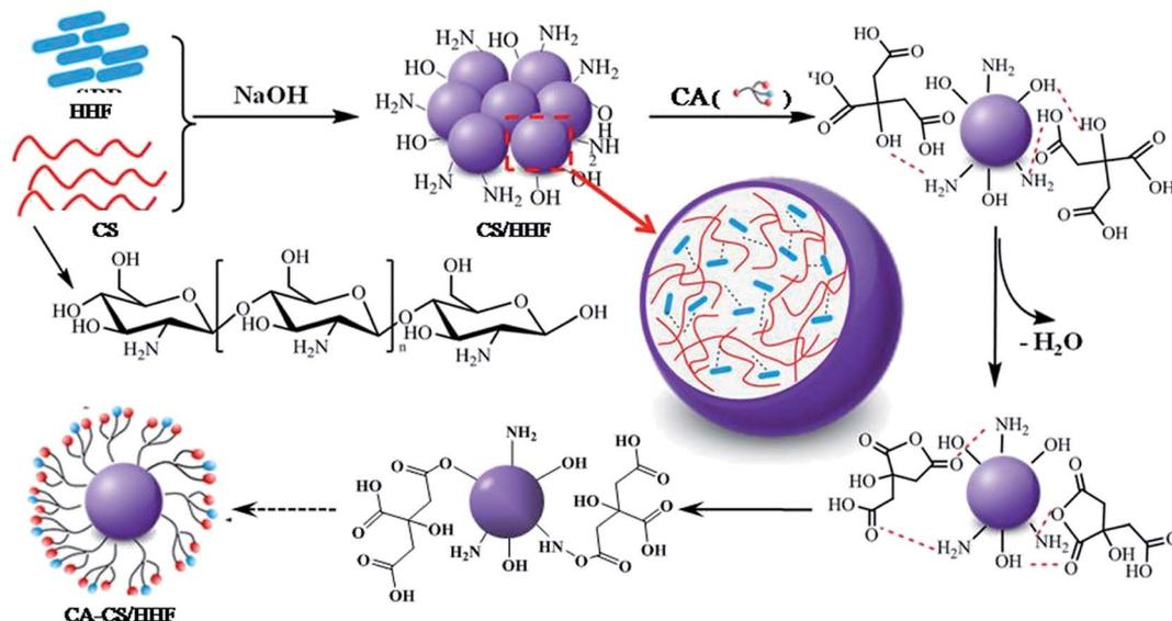
Scheme 1 Proposed mechanism for the formation of CA-CS/HHF hybrid beads.
