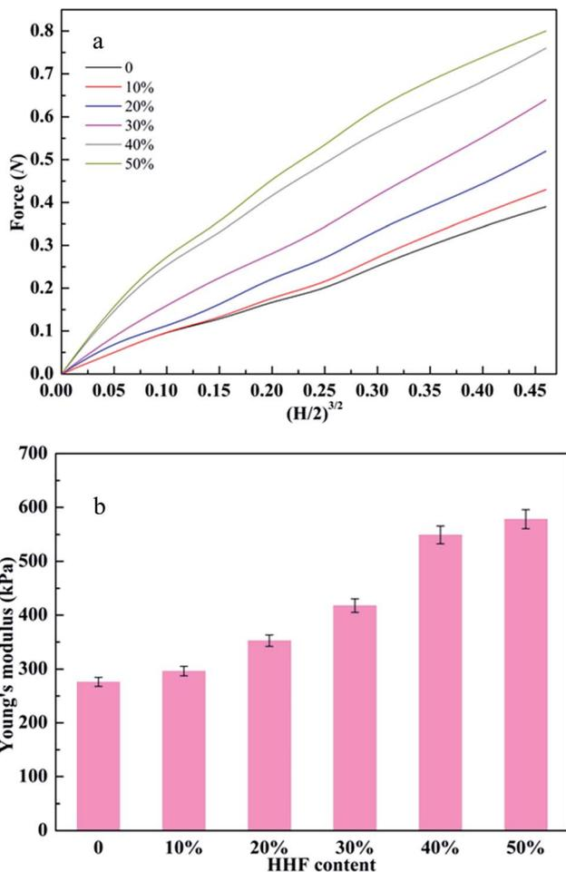
Fig. 3 (a) The force (N) and  $(H/2)^{3/2}$  curves of CA-CS/HHF composite beads with 40% final deformation;  $H$  is the displacement. (b) Effect of the HHF content on the Young's modulus of CA-CS/HHF composite beads.
