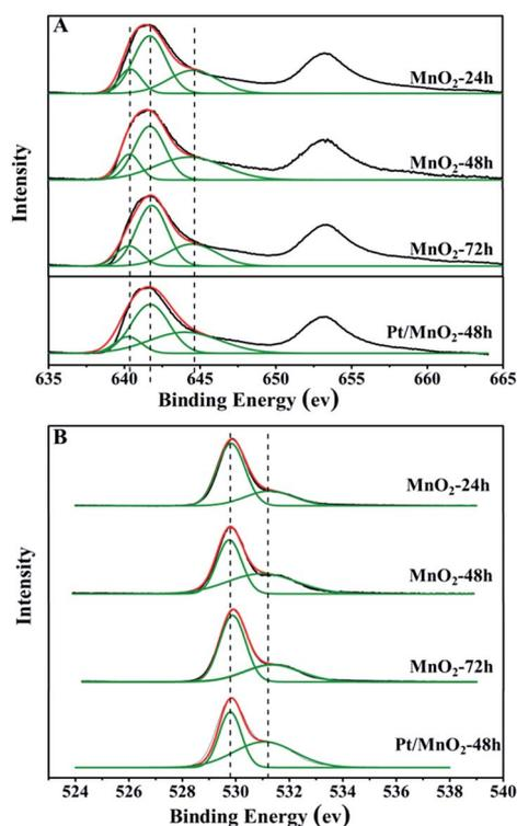
Fig. 5 XPS spectra of Mn 2p (A) and O 1s (B) of the as-synthesized MnO<sub>2</sub> and Pt/MnO<sub>2</sub>-48 h catalysts.
