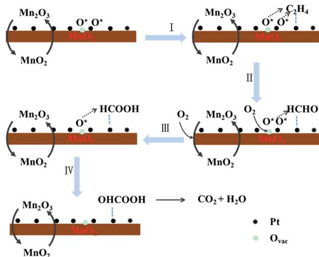
Fig. 9 The possible mechanism of C<sub>2</sub>H<sub>4</sub> catalytic oxidation on Pt/MnO<sub>2</sub>.
