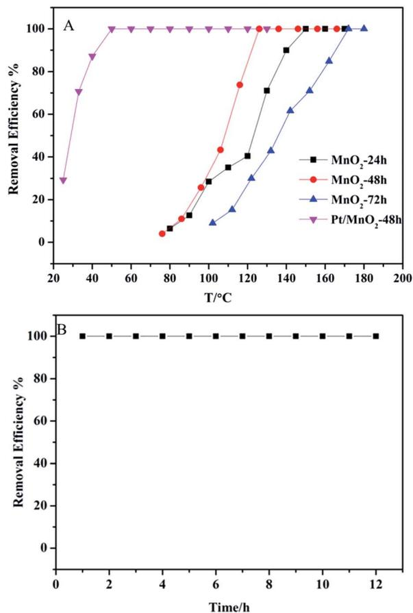
Fig. 8 (A) C<sub>2</sub>H<sub>4</sub> removal efficiency of by the as-synthesized MnO<sub>2</sub> and Pt/MnO<sub>2</sub>-48 h as functions of temperature; (B) C<sub>2</sub>H<sub>4</sub> removal efficiency by Pt/MnO<sub>2</sub>-48 h at 50 °C. Reaction condition: [C<sub>2</sub>H<sub>4</sub>] = 20 ppm, O<sub>2</sub> = 20.0 vol%, N<sub>2</sub> balance, GHSV = 60 000 mL g<sup>-1</sup> h<sup>-1</sup>.
