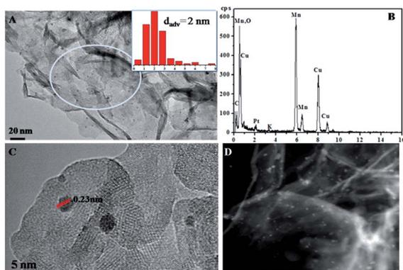
Fig. 4 The TEM image (A) (insert: the size distribution of Pt), EDS spectra (B), HRTEM image (C) and HADDF TEM image (D) of Pt/MnO<sub>2</sub>-48 h.
