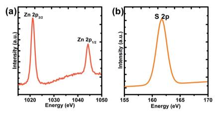
Fig. 2 XPS spectrum of the ZnS spheres prepared without the addition of PVP. (a) Zn 2p; (b) S 2p.
