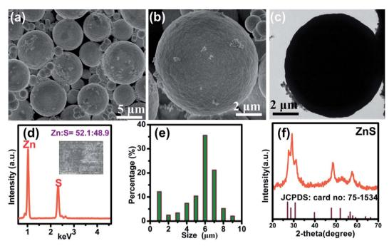
Fig. 1 (a and b) FE-SEM images (c) the TEM image of the ZnS prepared without PVP; (d) EDS spectrum (e) and size distribution of these ZnS micrometer spheres without the addition of PVP. (f) XRD patterns of the ZnS without PVP.
