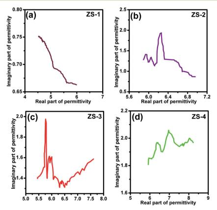
Fig. 7 Cole-Cole curves of the ZnS samples.
