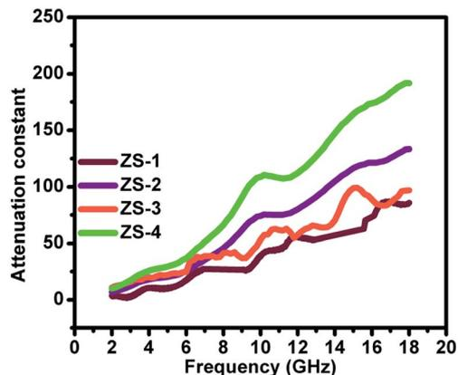
Fig. 6 Attenuation constant of the ZnS samples.
