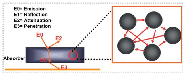
Fig. 8 Illustration of the scattering effect mechanism.
