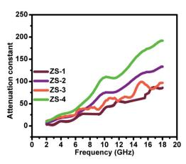
Fig. 6 Attenuation constant of the ZnS samples
