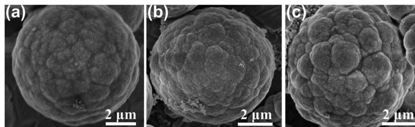
Fig. 3 FE-SEM images of the ZnS spheres with various amounts of PVP: (a) 10 mg; (b) 20 mg; (c) 30 mg.
