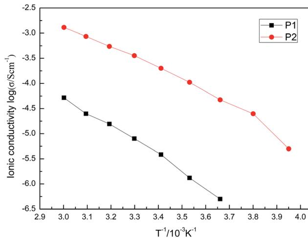
Fig. 11 Temperature dependence of polymer P1 and P2.
