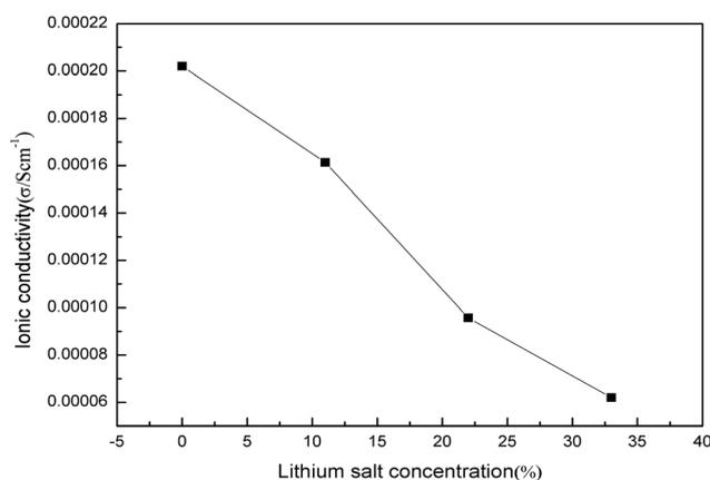
Fig. 13 Lithium salt concentration dependence of P2.
