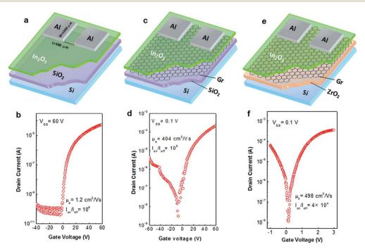
Fig. 6 Schematic illustration of the fabrication of different TFTs and the corresponding transfer characteristics. (a, b) pristine  $In_2O_3$  TFT, (c, d)  $In_2O_3$ /graphene TFT, and (e, f)  $In_2O_3$ /graphene TFT on high-k ZrO<sub>2</sub>.
