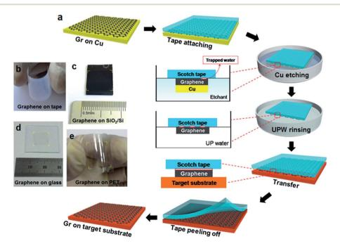
Fig. 1 (a) Schematic representation of transferring graphene from copper foil to target substrates. Photographs of graphene films transferred onto (b) scotch tape, (c) SiO<sub>2</sub>/Si, (d) glass and (e) PET. (Gr refers to graphene.)
