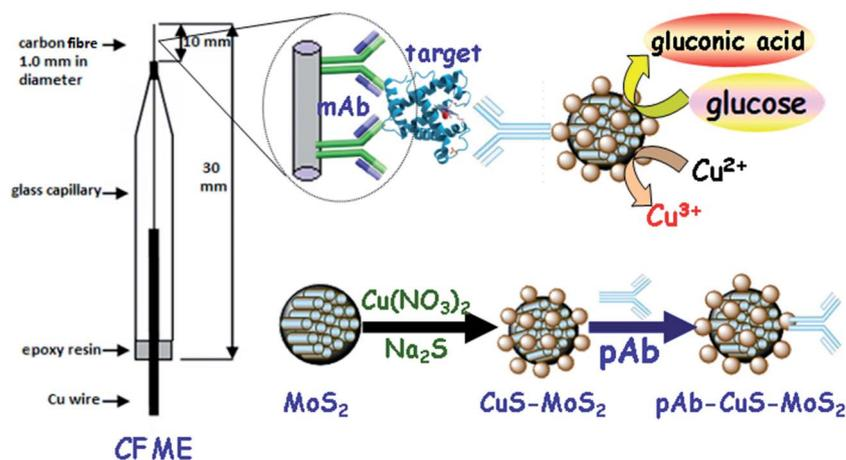
**Scheme 1** Schematic illustration of the CuS- $\text{MoS}_2$ -based, enzyme-free, electrochemical immunoassay of the target myoglobin on monoclonal mouse anti-myoglobin capture antibody (mAb)-modified carbon fiber microelectrode (CFME), using polyclonal rabbit anti-myoglobin detection antibody (pAb)-conjugated CuS- $\text{MoS}_2$  hybrid nanostructures as the signal-generation tags for glucose oxidation.
