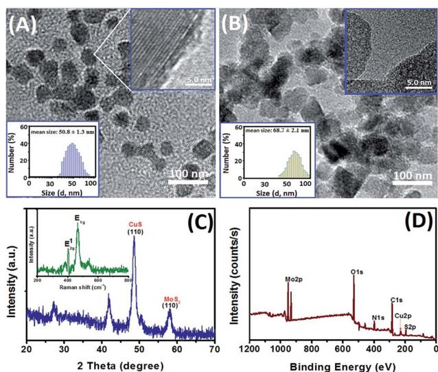
Fig. 1 HRTEM images of (A) MoS<sub>2</sub> nanocrystals and (B) CuS–MoS<sub>2</sub> hybrid nanostructures [inset: (top) magnification images and (bottom) DLS data of the corresponding nanostructures]. (C) XRD patterns (inset: Raman spectrum of CuS–MoS<sub>2</sub> hybrid nanostructures with the lowest laser power). (D) XPS data of CuS–MoS<sub>2</sub> nanostructures.
