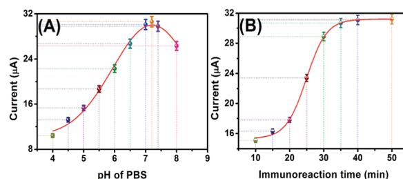
Fig. 3 Effects of (A) pH of PBS and (B) immunoreaction time of mAb-CFME with target myoglobin and pAb-CuS-MoS<sub>2</sub> on the anodic current of the electrochemical immunosensor (10 ng mL<sup>-1</sup> myoglobin used in this case).
