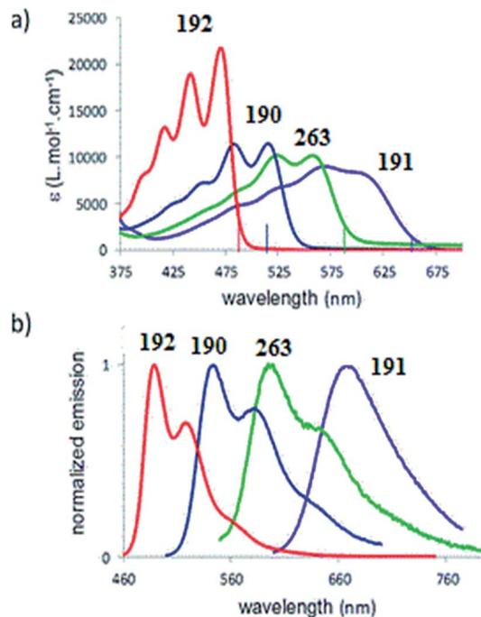
**Fig. 5** UV-Vis absorption spectra (a), normalised emission spectra (b) of the compounds **190–192** and **263** in dichloromethane ( $10^{-5}$  M)<sup>49</sup> (reprinted with permission from the American Chemical Society).
