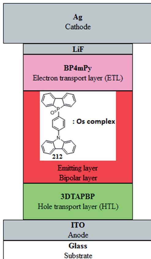
Fig. 6 Three-layer OLED.
