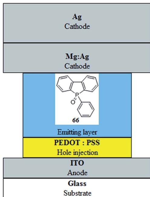
Fig. 8 Single-layer OLEDs.
