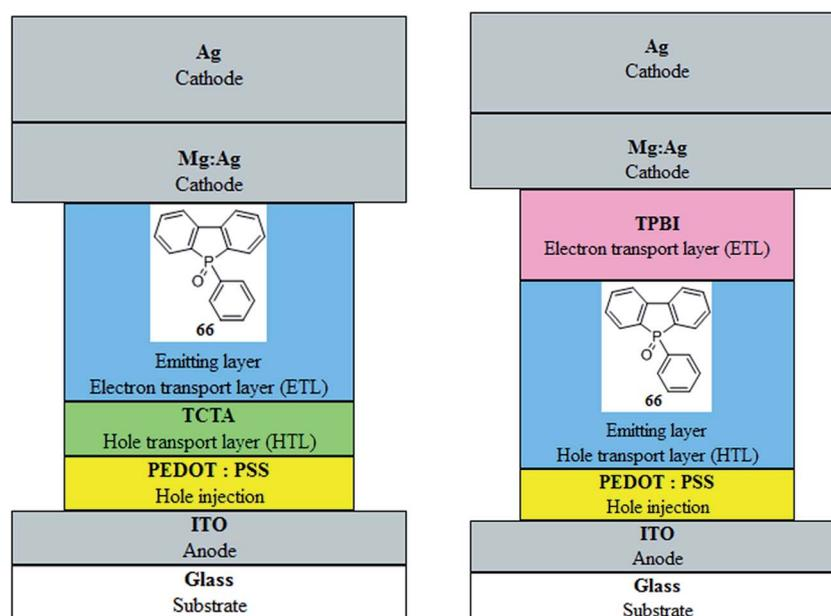
Fig. 9 Two-layer OLEDs.
