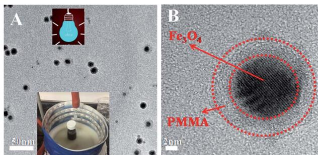
Fig. 2 Representative TEM characterization results of core/shell Fe<sub>3</sub>O<sub>4</sub>/PMMA with different scale bars. (A) 20 nm; (B) 2 nm. Inset: representative configuration comprising reaction vial surrounded by 380 nm LEDs with a tube blowing compressed air for cooling.
