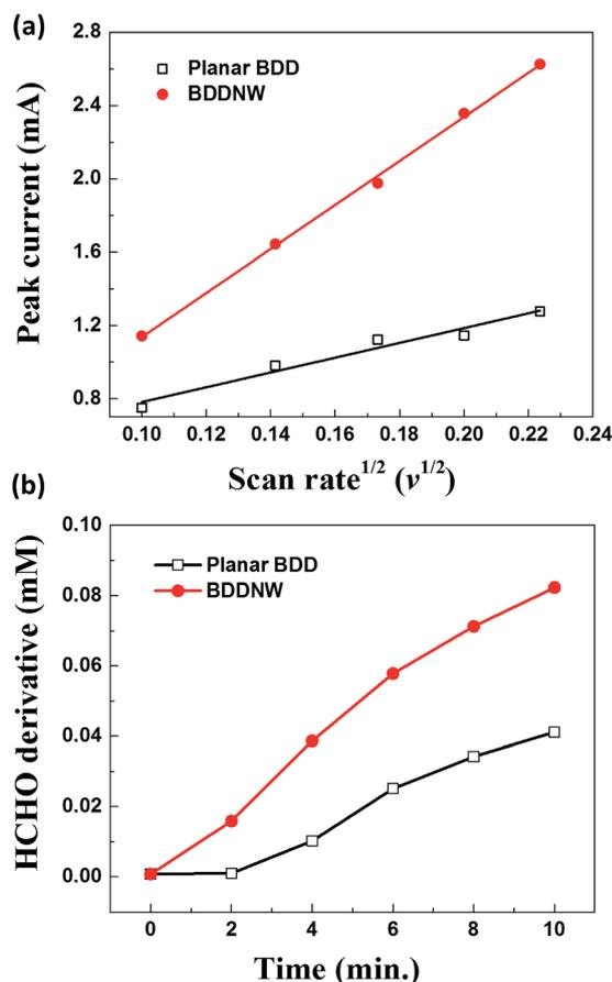
Fig. 4 (a) Peak current versus the square root of the scan rate and (b) formaldehyde produced by reacting  $\cdot\text{OH}$  with methanol.
