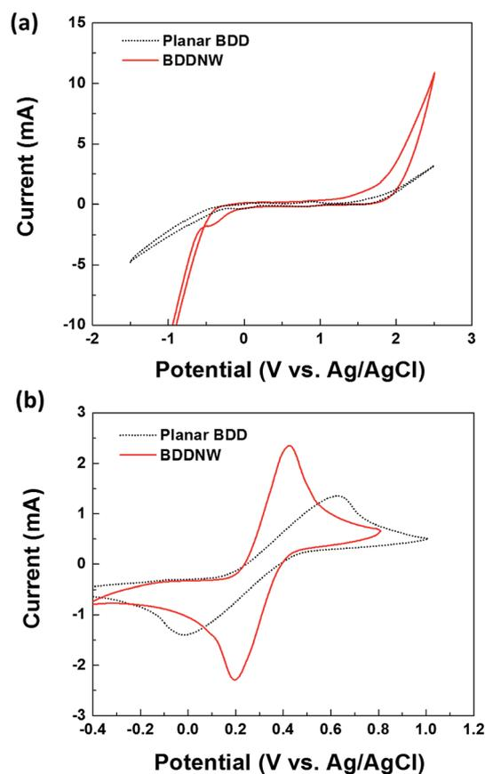
Fig. 3 Cyclic voltammograms of planar BDD and BDDNW electrodes in (a) 0.5 M  $\text{H}_2\text{SO}_4$  and (b) 3 M KCl solution containing 10 mM  $\text{Fe}(\text{CN})_6^{3-/4-}$ ; the voltammograms were collected using a scan rate of 50  $\text{mV s}^{-1}$ .
