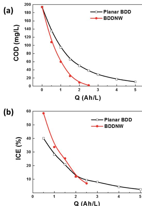
Fig. 5 (a) COD and (b) ICE curves for phenol oxidation on different electrodes.
