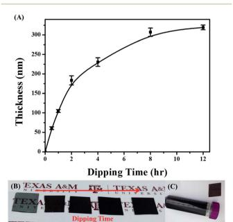
Fig. 1 The growth of PPy coating. (A) Growth of PPy coating on glass substrate with increased dipping time from 0.5 h to 12 h (B) PPy coating on the glass with the increasing dipping time (left to right: 0.5 h, 1 h, 4 h, 8 h, and 12 h). (C) PPy coating on glass and polypropylene plastic tube after 12 h.
