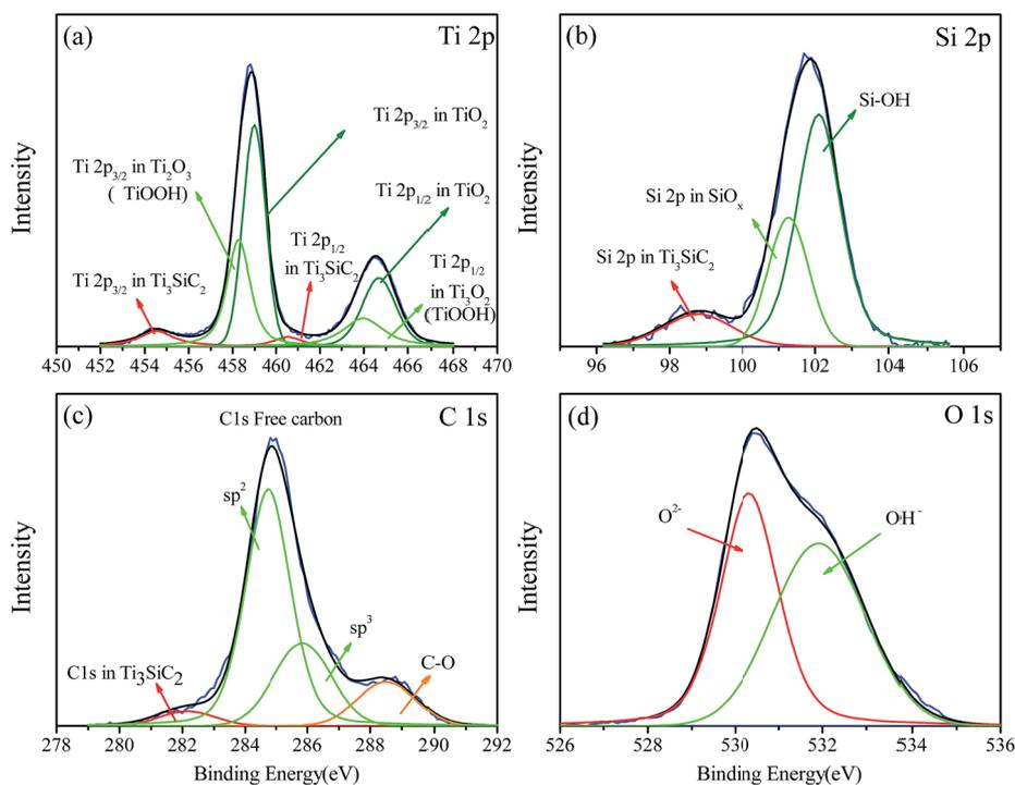
Fig. 4 Deconvoluted XPS spectra recorded at the layer formed on  $\text{Ti}_3\text{SiC}_2$  potentiostatically polarized at 1.25 V in 3.5% NaCl solution for 12 hours, (a) Ti 2p, (b) Si 2p, (c) C 1s, (d) O 1s.
