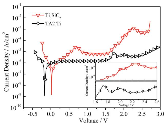
Fig. 1 Potentiodynamic polarization curves of  $\text{Ti}_3\text{SiC}_2$  and commercial titanium (CP Ti) in 3.5% NaCl solution at scanning rate of 0.333 mV s<sup>-1</sup>.
