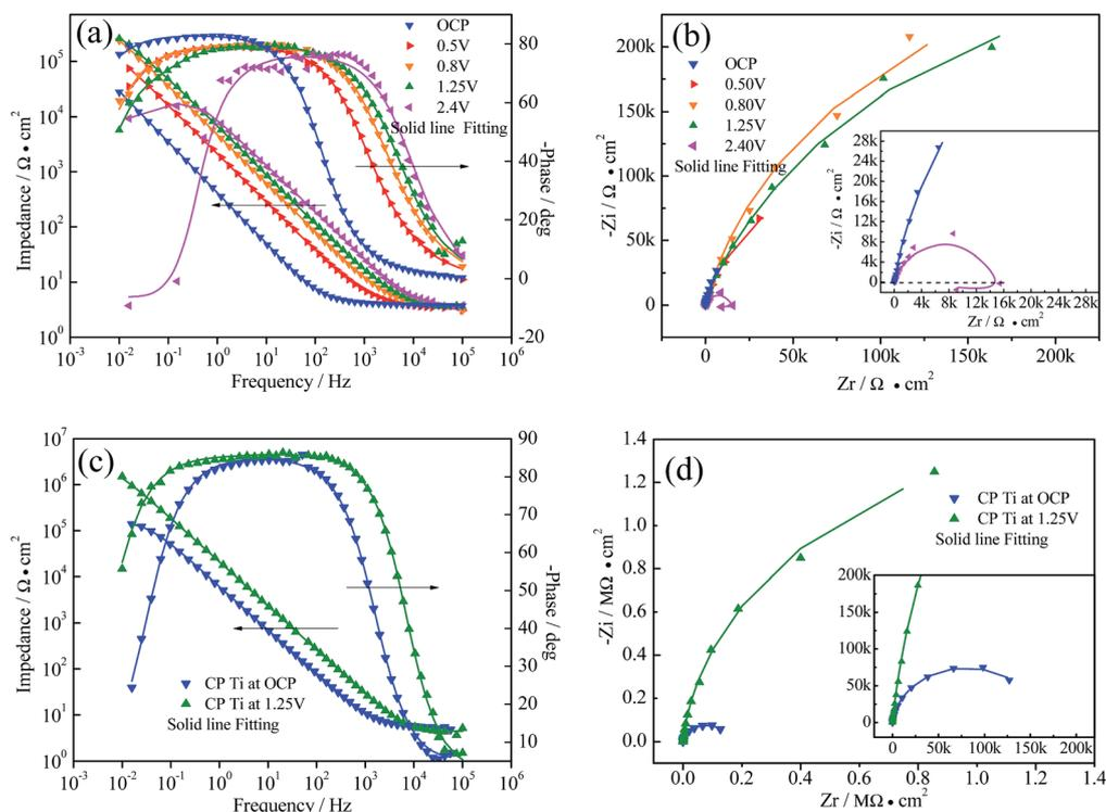
**Fig. 2** Electrochemical impedance spectroscopy of Ti<sub>3</sub>SiC<sub>2</sub> and CP Ti in 3.5% NaCl solution after immersion for 30 min (OCP) and potentiostatic polarization for 12 hours at different potential, (a) Bode plot of Ti<sub>3</sub>SiC<sub>2</sub>, (b) Nyquist plot of Ti<sub>3</sub>SiC<sub>2</sub>, (c) Bode plot of CP Ti, and (d) Nyquist plot of CP Ti.
