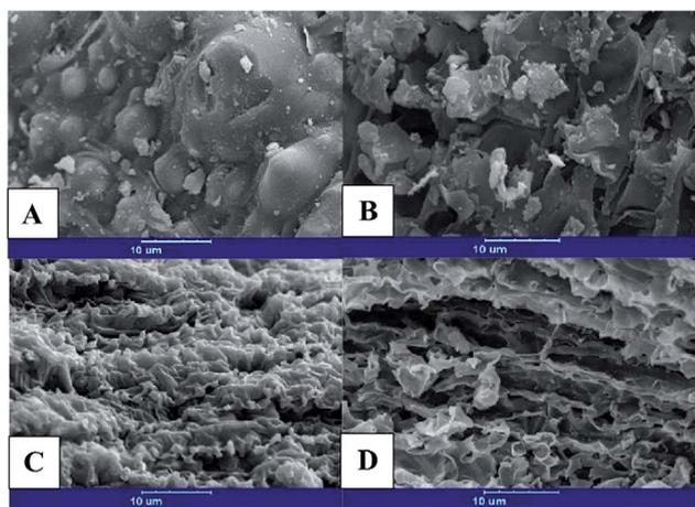
**Fig. 2** SEM image (1000× magnification) of (A) untreated rice straw (B) pretreated rice straw with 2 M NaOH at 0 °C for 150 min (C) pretreated rice straw with 0.5 M NaHCO<sub>3</sub> at 180 °C for 180 min (D) pretreated rice straw with 2 M NaOH at 100 °C for 120 min.
