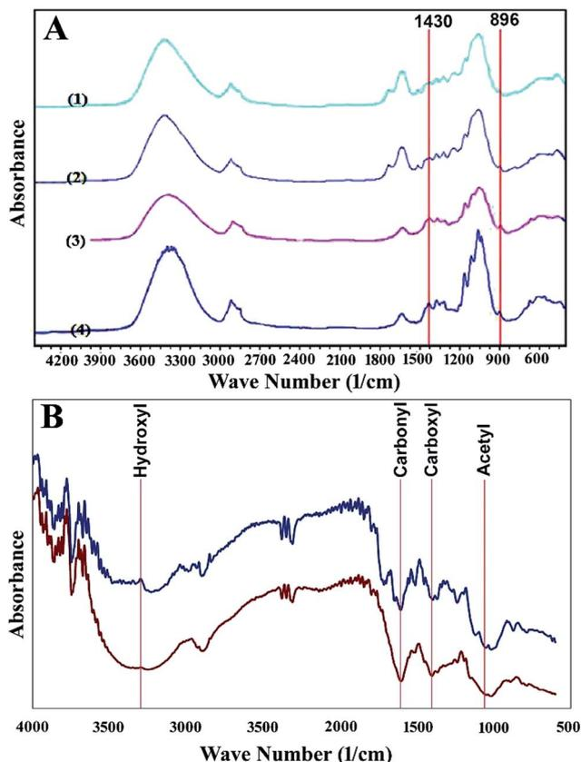
**Fig. 1** (A) The FTIR of (1) untreated rice straw, (2) pretreated rice straw with 2 M NaOH at 0 °C for 150 min, (3) pretreated rice straw with 0.5 M NaHCO<sub>3</sub> at 180 °C for 180 min and (4) pretreated rice straw with 2 M NaOH at 100 °C for 120 min. (B) The FTIR spectra of (1) produced xanthan and (2) commercial xanthan.
