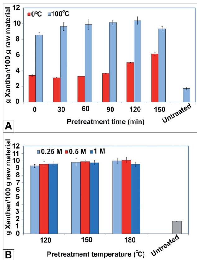
Fig. 4 Xanthan yield obtained from (A) pretreatment with 2 M NaOH at 0 °C and 100 °C and (B) pretreatment with NaHCO<sub>3</sub> at different concentrations and temperatures.
