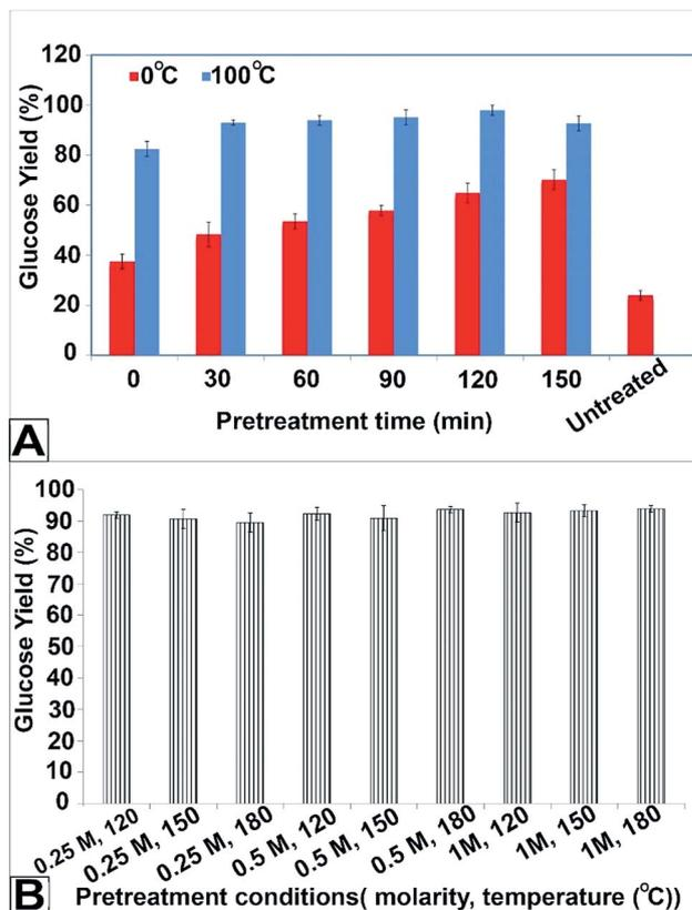
**Fig. 3** Glucose yield obtained from (A) pretreatment with 2 M NaOH at 0 °C, (B) pretreatment with 2 M NaOH at 100 °C.
