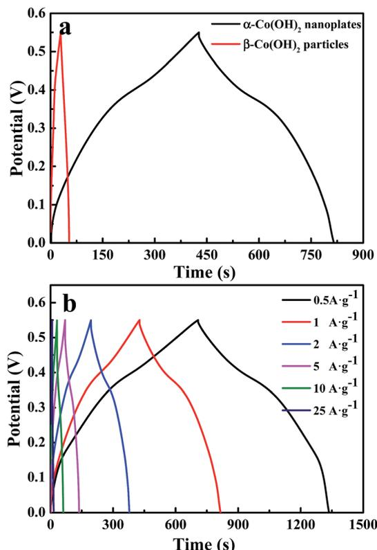
Fig. 6 Charge-discharge curves in a three-electrode system of (a)  $\alpha$ -Co(OH)<sub>2</sub> nanoplates and  $\beta$ -Co(OH)<sub>2</sub> particles at a charge-discharge current density of 1 A g<sup>-1</sup> and (b)  $\alpha$ -Co(OH)<sub>2</sub> nanoplates at different current densities.
