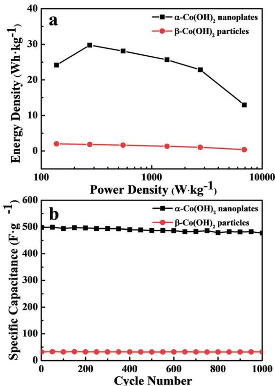
Fig. 7 (a) Ragone plot of the electrode made from the samples at different current densities and (b) cycling properties of the samples at current density of 5 A g<sup>-1</sup>.
