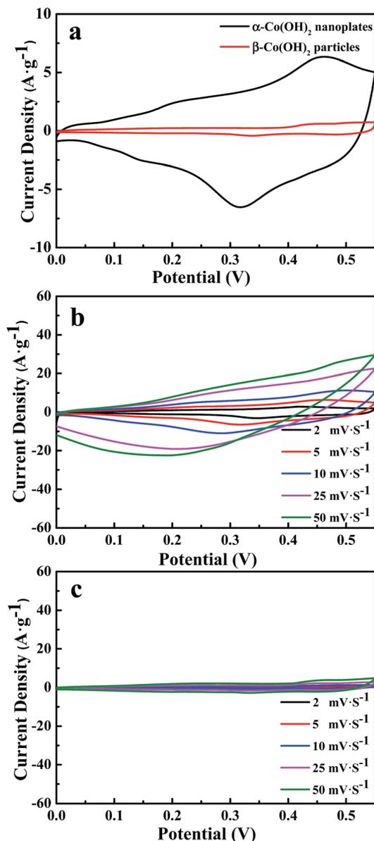
Fig. 5 CV curves in a three-electrode system of (a)  $\alpha$ -Co(OH)<sub>2</sub> nanoplates and  $\beta$ -Co(OH)<sub>2</sub> particles at a scanning rate of 5 mV s<sup>-1</sup>, (b)  $\alpha$ -Co(OH)<sub>2</sub> nanoplates at a scanning rate of 2–50 mV s<sup>-1</sup> and (c)  $\beta$ -Co(OH)<sub>2</sub> particles at a scanning rate of 2–50 mV s<sup>-1</sup>.
