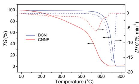
Fig. 4 TGA curves of BCN and CNNF at a heating rate of 10 °C min<sup>-1</sup> under air flux.
