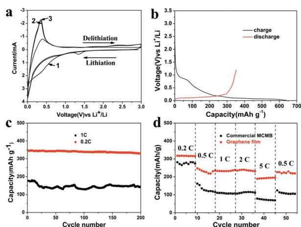
Fig. 3 (a) Cyclic voltammetry profiles of the as-obtained graphene film at a  $1\text{ mV s}^{-1}$  scan rate (voltage range: 0.01–3.0 V) and (b) galvanostatic charge–discharge curves for the first cycle cycled between 0.01 V and 1.2 V versus  $\text{Li}^+/\text{Li}$  at 0.1C. (c) Cycling performance of the as-obtained graphene film at different current densities and (d) rate capability of the as-obtained graphene film and the commercial MCMB/copper system.
