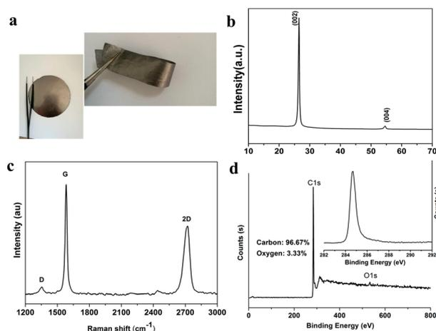
Fig. 2 (a) Optical image, (b) XRD patterns, (c) Raman spectra and (d) XPS spectra of the as-prepared graphene film.
