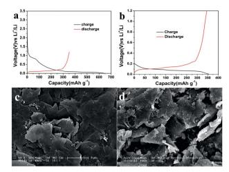
Fig. 4 Galvanostatic charge—discharge curves for the first cycle between 0.01 V and 1.2 V *versus* Li<sup>+</sup>/Li at 0.1C of the as-obtained graphene film before (a) and after (b) surface treatment. SEM images of the film before (c) and after (d) surface treatment.
