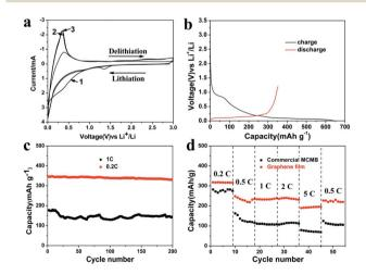
Fig. 3 (a) Cyclic voltammetry profiles of the as-obtained graphene film at a 1 mV s<sup>-1</sup> scan rate (voltage range: 0.01-3.0 V) and (b) galvanostatic charge-discharge curves for the first cycle cycled between 0.01 V and 1.2 V versus Li<sup>+</sup>/Li at 0.1C. (c) Cycling performance of the as-obtained graphene film at different current densities and (d) rate capability of the as-obtained graphene film and the commercial MCMB/copper system.
