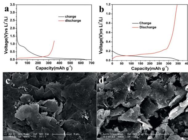
Fig. 4 Galvanostatic charge-discharge curves for the first cycle between  $0.01 \text{ V}$  and  $1.2 \text{ V}$  versus  $\text{Li}^+/\text{Li}$  at  $0.1\text{C}$  of the as-obtained graphene film before (a) and after (b) surface treatment. SEM images of the film before (c) and after (d) surface treatment.
