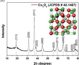
Fig. 1 Synthesis of Co<sub>3</sub>O<sub>4</sub> nanoparticles. XRD patterns of (a) commercially available CoO(OH) powder and (b) Co<sub>3</sub>O<sub>4</sub> obtained by mechanochemical transformation of CoO(OH) powder. The crystalline structure of Co<sub>3</sub>O<sub>4</sub> is also shown as inset in (b).
