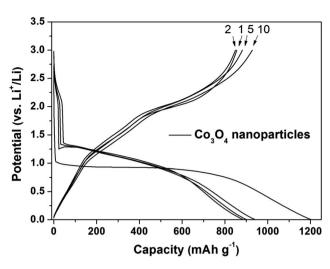
Fig. 3 Electrochemical performance of  $Co_3O_4$  nanoparticles electrode. Galvanostatic voltage profile of  $Co_3O_4$  nanoparticles electrode (current density: 100 mA  $g^{-1}$ , voltage window: 0.0–3.0 V).
