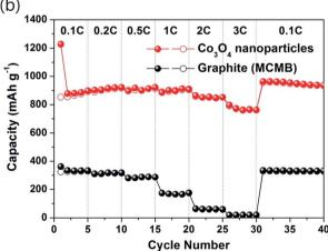
Fig. 6 Cycling performance and rate capability of  $Co_3O_4$  nanoparticles electrode. (a) Cycling performance of the  $Co_3O_4$  nanoparticles electrode and an MCMB-graphite electrode at a cycling rate of 100 mA  $g^{-1}$ , and (b) rate capabilities of the  $Co_3O_4$  nanoparticles electrode and an MCMB-graphite electrode at various C rates.
