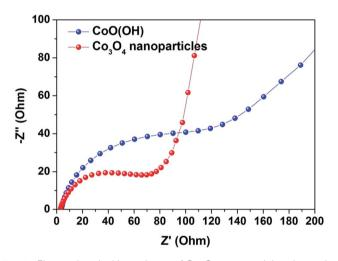
Fig. 4 Electrochemical impedance of  $Co_3O_4$  nanoparticles electrode. Electrochemical Nyquist plots of CoO(OH) and  $Co_3O_4$  nanoparticles electrodes.
