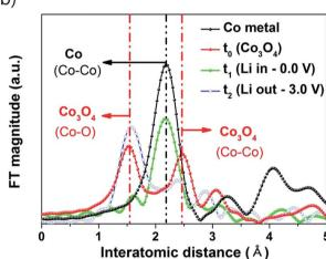
Fig. 5 Electrochemical reaction mechanism of  $\text{Co}_3\text{O}_4$  nanoparticles electrode. (a) DCP for the first and second cycling and (b) Co K-edge EXAFS results during the first cycle for  $\text{Co}_3\text{O}_4$  nanoparticles electrode.
