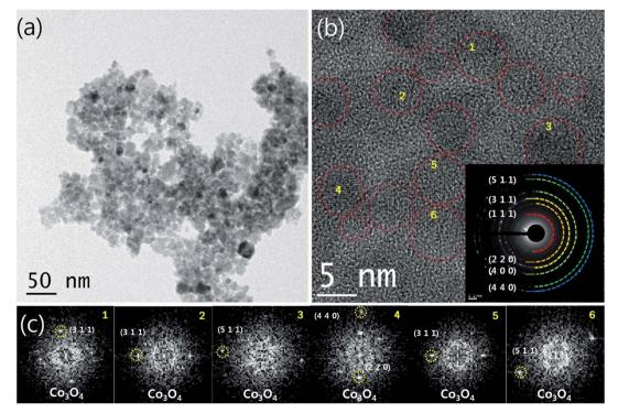
Fig. 2 Morphological investigation of Co<sub>3</sub>O<sub>4</sub> nanoparticles. (a) TEM bright-field and (b) HRTEM images with their corresponding SAED and (c) FT patterns for synthesized Co<sub>3</sub>O<sub>4</sub> nanoparticles
