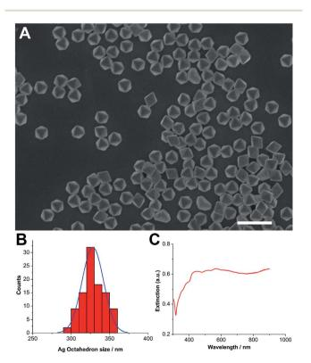
Fig. 1 Characterization of Ag octahedrons. (A) Representative scanning electron microscopy image of synthesized Ag octahedral nanoparticles. Scale bar, 1  $\mu$ m. (B) Size distribution of Ag octahedral nanoparticles (n > 500) measured from SEM images. (C) Extinction spectra of Ag octahedral nanoparticles.
