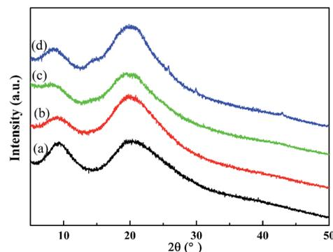
Fig. 2 XRD patterns of wool keratin (a) and keratin regenerated from [DBNE]DEP (b), [Emim]DEP (c), and [DBNH]OAc (d) solutions.
