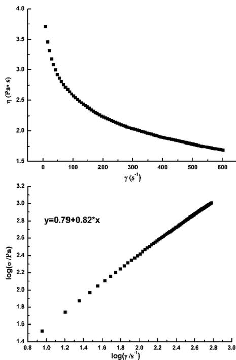
Fig. 10 Dependence of the apparent viscosity on the shear rate and the logarithmic plots of shear stress vs. shear rate of a [DBNE]DEP solution at a mass ratio of 8 wt% and temperature of 333 K.
