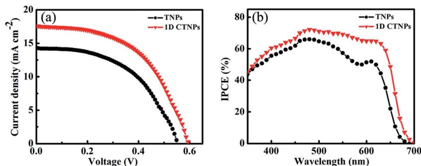
Fig. 5 (a)  $J$ - $V$  characteristics and (b) IPCE spectra of QDSSCs based on TNPs and 1D CTNPs films.
