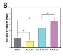
Fig. 4 Mechanical properties of the pure PLGA, PLGA–Gel, and GO–PLGA and GO–PLGA–Gel nanofibrous matrices tested at room temperature. (A) Typical stress–strain curves, (B) tensile strength. (n = 3; \*p < 0.05).
