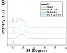
Fig. 2 (A) FTIR spectra of PLGA, PLGA–Gel, GO–PLGA and GO–PLGA–Gel nanofibrous matrices. (B) XRD patterns of powdery GO, PLGA, PLGA–Gel, GO–PLGA and GO–PLGA–Gel nanofibrous matrices.
