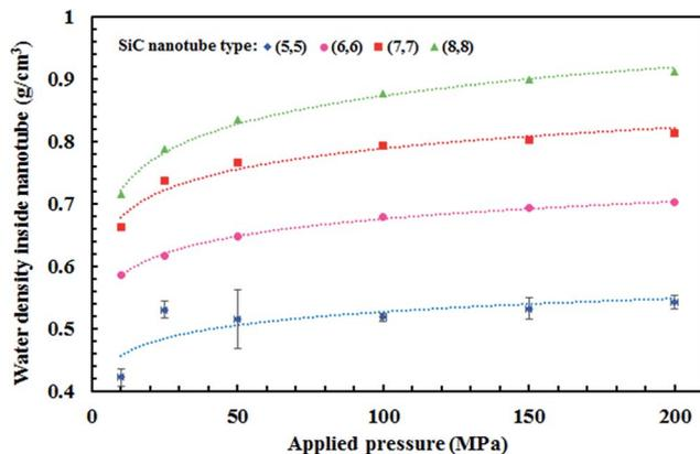
Fig. 5 Density of water molecules inside SiC nanotubes of different diameters and at different pressures. Error bars represent the uncertainty of the corresponding data and are only shown for values greater than the data points.
