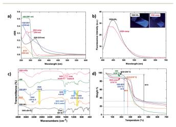
Fig. 1 Characterization of GQD-NH<sub>2</sub>, GQD- $\beta$ CD, and GQD-comp using UV/Vis spectroscopy (a), fluorescence spectroscopy (b), FTIR (c), and TGA (d). Blue-color emission of GQD-NH<sub>2</sub> and GQD-comp were observed under the UV lamp (365 nm) (b, inset).
