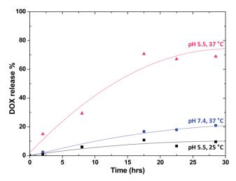
Fig. 4 In vitro release profile of DOX from DL-GQD in PBS under different conditions: pH 5 at 37 °C, pH 7.4 at 37 °C, and pH 5 at 25 °C.
