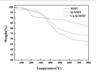
Fig. 7 TGA curves of MMT, Q-MMT and Cu-Q-MMT.
