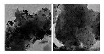
Fig. 5 TEM micrographs of virgin Cu-Q-MMT (left) and the recycled Cu-Q-MMT (right).
