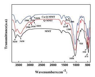
Fig. 2 FTIR analysis of MMT, Q-MMT and Cu-Q-MMT.
