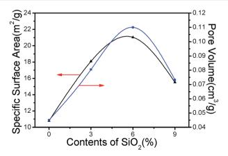
Fig. 12 Effect of SiO<sub>2</sub> content on SiO<sub>2</sub>/PS fibers SSA and pore volume.
