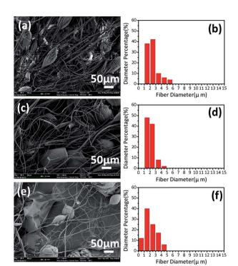
Fig. 5 SEM images and fiber diameter distributions of PS fibers centrifugally-spun from the 16 wt% solution at 8000 rpm using a nozzle with 0.4 mm diameter and different nozzle-collector distances: (a and b) 6 cm, (c and d) 9 cm, and (e and f) 12 cm.
