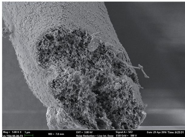
Fig. 11 SEM image of 9 wt% SiO<sub>2</sub>/PS fiber cross-section.
