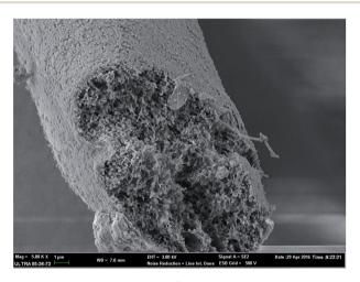
Fig. 11 SEM image of 9 wt% SiO<sub>2</sub>/PS fiber cross-section.
