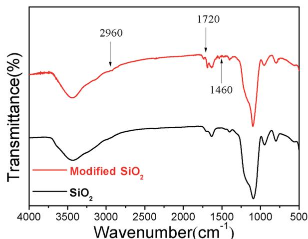
Fig. 7 FTIR-ATR spectra of SiO<sub>2</sub> before and after modification.
