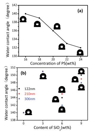
Fig. 9 WCA and the corresponding shapes of water droplets for the PS fibers centrifugally-spun from (a) different PS solution concentrations and (b) 16 wt% solution at 8000 rpm using a nozzle with diameter of 0.4 mm and nozzle-collector distance of 12 cm, with different particle size and SiO<sub>2</sub> content.
