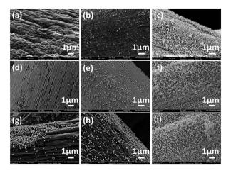
Fig. 8 SEM images of SiO<sub>2</sub>/PS fibers centrifugally-spun from 16 wt% solution at 8000 rpm using nozzle diameter of 0.4 mm and nozzlecollector distance of 12 cm with different SiO<sub>2</sub> particle sizes: (a)–(c) 122 nm; (d)-(f) 210 nm; (g)-(i) 306 nm; and concentrations: (a), (d) and (g) 3 wt%, (b), (e) and (f) 6 wt%, (c), (f) and (i) 9 wt%.
