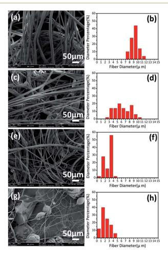
Fig. 3 SEM images and fiber diameter distributions of PS fibers centrifugally-spun from a 16 wt% solution using a 0.4 mm nozzle and a 12 cm nozzle-collector distance at different rotational speeds: (a and b) 5000 rpm, (c and d) 6000 rpm, and (e and f) 7000 rpm, (g and h) 8000 rpm.
