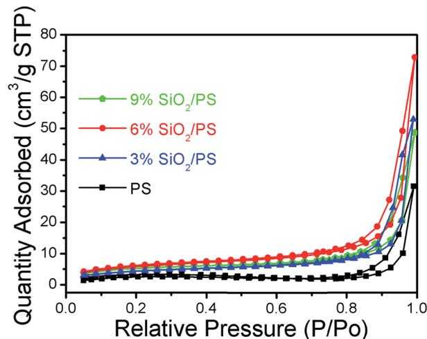
Fig. 13 Nitrogen adsorption/desorption isotherms of SiO<sub>2</sub>/PS fibers.
