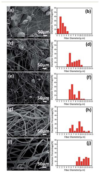
Fig. 2 SEM images and fiber diameter distributions of PS fibers centrifugally-spun at 8000 rpm using a 0.4 mm nozzle and a 12 cm nozzle-collector distance with different solution concentrations: (a and b) 16 wt%, (c and d) 18 wt%, (e and f) 20 wt%, (g and h) 22 wt%, and (i and j) 24 wt%.
