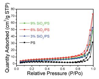
Fig. 13 Nitrogen adsorption/desorption isotherms of SiO<sub>2</sub>/PS fibers.
