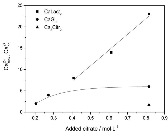
Fig. 3 Calcium citrate supersaturation expressed as a degree of supersaturation  $Ca^{2+}_{max}/Ca^{2+}_{eq}$  after adding solid sodium citrate to calcium L-lactate, calcium D-gluconate, or to calcium citrate.
