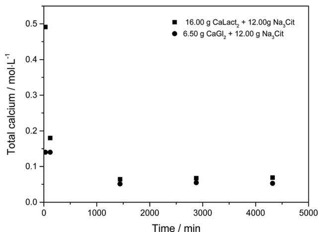
**Fig. 1** Calcium concentration in 100 mL of water during dissolution of 16.00 g of solid calcium L-lactate mixed with 12.00 g of sodium citrate, and of 6.50 g of calcium D-gluconate mixed with 12.00 g of sodium citrate under constant stirring at 25 °C, followed by precipitation of calcium citrate.
