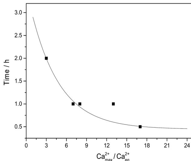
Fig. 4 Lag phase for initiation of precipitation of calcium citrate in supersaturated solutions made by dissolution of calcium L-lactate by sodium citrate in water at 25 °C.  $Ca^{2+}_{max}/Ca^{2+}_{eq}$  is the degree of supersaturation determined by titration of  $Ca^{2+}$  in maximal supersaturated solution. Curve is based on fitting to an exponential equation to yield:  $time = 3.09 \exp(-Ca^{2+}_{max}/Ca^{2+}_{eq}/4.33) + 0.44$  (all points except point for supersaturation degree of 12).
