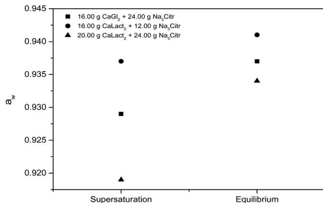
Fig. 2 Water activity,  $a_w$ , of supersaturated and equilibrated solutions of calcium citrate at 25 °C made by dissolution of calcium L-lactate and sodium citrate or by dissolution of calcium D-gluconate and sodium citrate in 100 mL of water.
