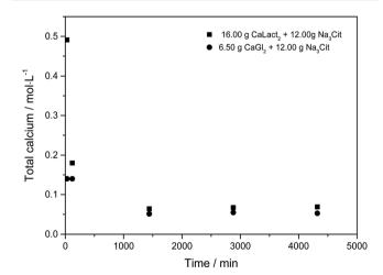
Fig. 1 Calcium concentration in 100 mL of water during dissolution of 16.00 g of solid calcium L-lactate mixed with 12.00 g of sodium citrate, and of 6.50 g of calcium p-gluconate mixed with 12.00 g of sodium citrate under constant stirring at 25 °C, followed by precipitation of calcium citrate.
