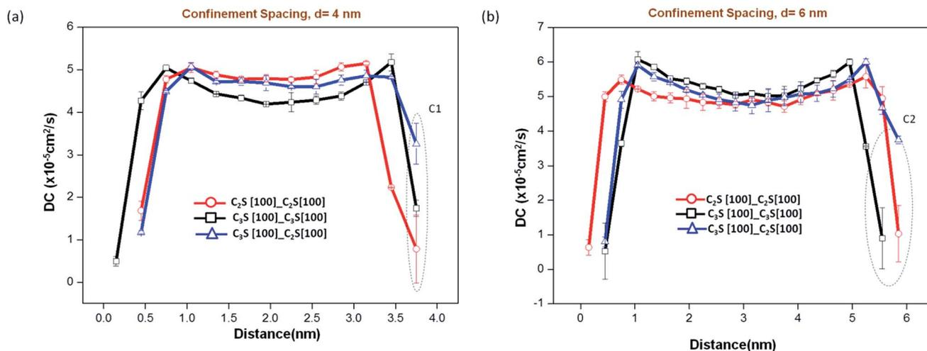
Fig. 6 Variation of diffusion coefficient across the water layer for different surface combinations and confinement spacings (a)  $d = 4$  nm and (b)  $d = 6$  nm. Figures depict the variation in DC value across the water layer for similar surface combinations of  $C_2S-C_2S$  and  $C_3S-C_3S$  and dissimilar surface combination,  $C_3S-C_2S$ . The DC value is higher at the  $C_2S$  end for dissimilar surfaces.
