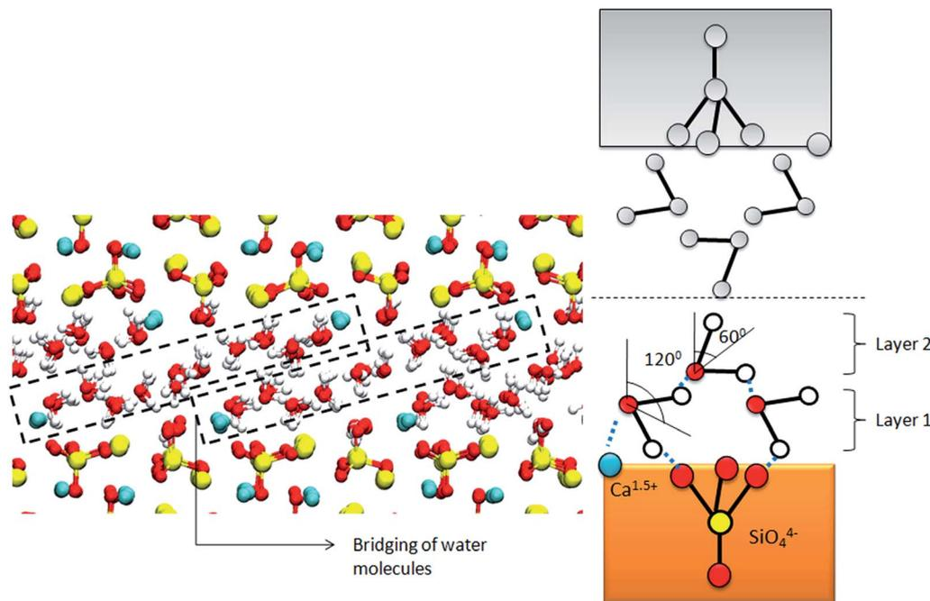
Fig. 5 Schematic showing structured water molecules throughout confinement volume for  $d = 10 \text{ \AA}$ . The layered structure of water is a result of the intermolecular H-bond network. The orientation profile exhibits two peaks at  $120^\circ$  and  $60^\circ$  respectively.
