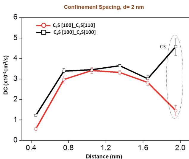
Fig. 7 Variation of diffusion coefficient of confined water with  $C_3S [1 0 0]$  as surface-1 and the cleavage planes of  $C_2S [1 0 0]$  and  $C_2S [1 1 0]$  as surface-2. At 2 nm confinement DC value of water molecules on  $C_2S [1 0 0]$  surface is raised whereas at  $[1 1 0]$  surface it is lowered.
