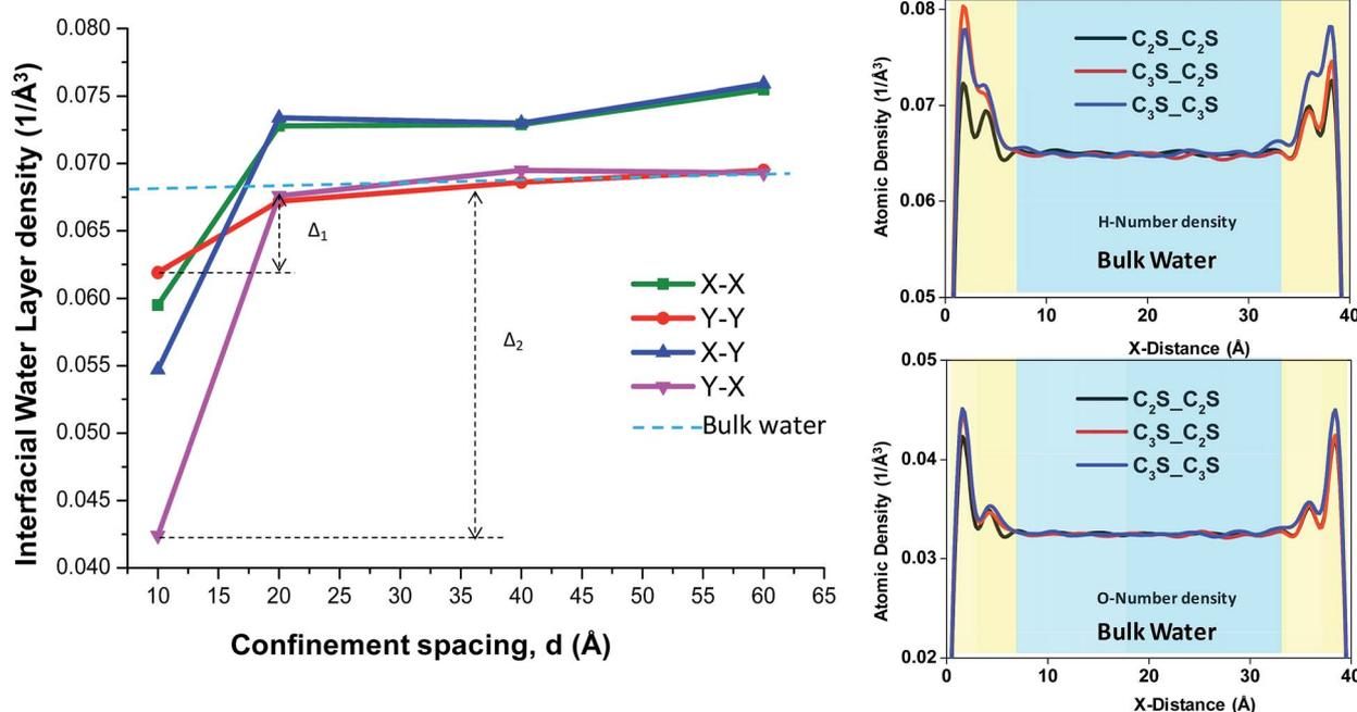
Fig. 3 The variation in maximum near-surface density of  $H_{\text{water}}$  vs. confinement spacing for different surface combinations. X-X and Y-Y represents the similar surface combinations and X-Y and Y-X represents the dissimilar surface combinations. In the inset, density profile of X-X, Y-Y and X-Y combination for a confinement spacing  $d = 40$  Å is also provided (X- $\text{C}_3\text{S}$  [1 0 0], Y- $\text{C}_2\text{S}$  [1 0 0]).
