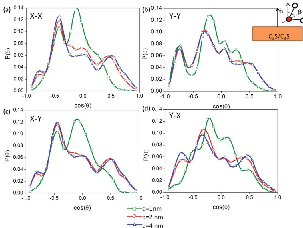
Fig. 4 The probability distribution of  $\cos(\theta)$  for water molecules on (a)  $C_3S$  surface in  $C_3S$ \_water\_ $C_3S$  system (b)  $C_2S$  surface in  $C_2S$ \_water\_ $C_2S$  system (c)  $C_3S$  surface in  $C_3S$ \_water\_ $C_2S$  system (d)  $C_2S$  surface in  $C_3S$ \_water\_ $C_2S$  system interfacial layer water molecules exhibit orientational bias or higher probability for certain fixed orientations (X– $C_3S$  [1 0 0], Y– $C_2S$  [1 0 0]).
