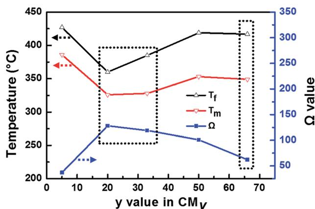
Fig. 5 The different characteristic temperatures ( $T_m$  and  $T_f$ ) and values of “ $\Omega$ ” as a function of  $y$  in  $\text{CM}_y$ . Reaction conditions for catalytic soot combustion: 500 ppm NO and 10%  $\text{O}_2$  in  $\text{N}_2$  with a total flow of  $200 \text{ mL min}^{-1}$ , mass of soot–catalyst–silica is 10–100–1000 mg, under loose contact mode.
