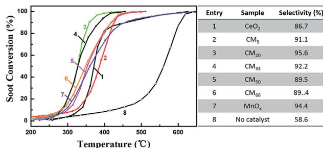
Fig. 1 Catalytic activity (left) and selectivity to CO<sub>2</sub> (right) for soot combustion over different catalysts or NULL (without catalyst) under loose contact mode. Reaction conditions: 500 ppm NO and 10% O<sub>2</sub> in N<sub>2</sub> with a total flow of 200 mL min<sup>-1</sup>, mass of soot–catalyst–silica is 10–100–1000 mg.
