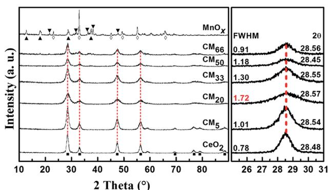
Fig. 2 XRD patterns of different  $\text{CM}_y$  composites and the references  $\text{MnO}_x$  and  $\text{CeO}_2$  (left), (■)- $\text{CeO}_2$ ; (◇)- $\text{Mn}_2\text{O}_3$ ; (▲)- $\text{MnO}_2$ ; (▼)- $\text{Mn}_5\text{O}_8$ ), and the enlarged region between  $25^\circ$  and  $31^\circ$  of the patterns showing the corresponding FWHM values and peak positions of  $2\theta$  (right).
