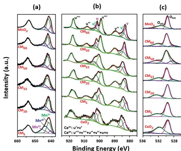
Fig. 4 XPS spectra of (a) Mn 2p, (b) Ce 3d and (c) O 1s for all CM<sub>y</sub> composites and the reference MnO<sub>x</sub> and/or CeO<sub>2</sub>.
