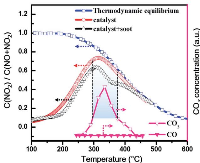
Fig. 7 The temperature-programmed oxidation of NO over CM<sub>33</sub> with or without soot under loose contact mode. Reaction conditions: 500 ppm NO and 10% O<sub>2</sub> in N<sub>2</sub> with a total flow of 200 mL min<sup>-1</sup>, the mass of (soot-)catalyst-silica is (10-)100–1000 mg.
