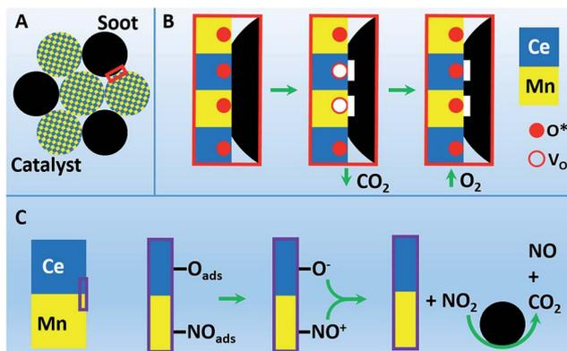
Scheme 1 Schematic illustration of (A) the sufficient mixing of  $\text{CM}_{20}$  and soot particles, and the possible pathways of soot combustion on  $\text{CM}_{20}$  in  $\text{NO}_x/\text{O}_2$ : (B) Route (i): direct soot combustion by surface active oxygen species; (C) Route (ii): NO-aided soot combustion.
