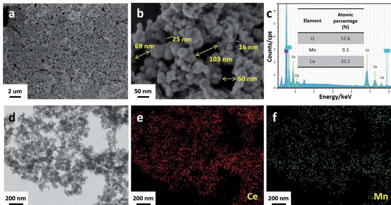
Fig. 3 Low-magnification SEM image (a), high-magnification SEM image (b), EDS spectrum (c), typical TEM image (d) and the element mapping (e and f) of CM<sub>20</sub>.
