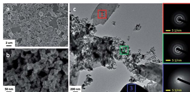
Fig. 6 Low-magnification SEM image (a), high-magnification SEM image (b), TEM image (c) of  $\text{CM}_{33}$ , and the corresponding SAED patterns to the different areas in (c).
