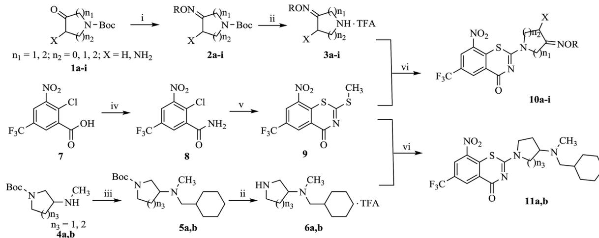
**Scheme 1** Synthesis of target compounds **10a–i** and **11a, 11b**. Reagents and conditions: (i)  $RONH_2 \cdot HCl$ ,  $K_2CO_3$ ,  $C_2H_5OH$ , rt, 40–65%; (ii) TFA,  $CH_2Cl_2$ , rt, 50–52%; (iii)  $c\text{-}C_6H_{11}CH_2Br$ ,  $K_2CO_3$ , DMF, 80 °C, 50–52%; (iv)  $SOCl_2$ ,  $NH_3 \cdot H_2O$ , reflux, 76%; (v)  $CS_2$ ,  $CH_3I$ , DMSO, rt, 41%; (vi)  $(C_2H_5)_3N$ ,  $C_2H_5OH$ , 60 °C, 45–59%.
