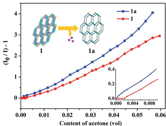
Fig. 5 The structure dependent sensing performances of **1** and **1a** presented by the relationship between quenching efficiency and acetone content in ethanol calculated from emission at 621 nm. The  $I_0$  and  $I$  present for the initial and quenched intensity of emission, respectively. The inset represents the quenching performances of **1** and **1a** at low concentration.
