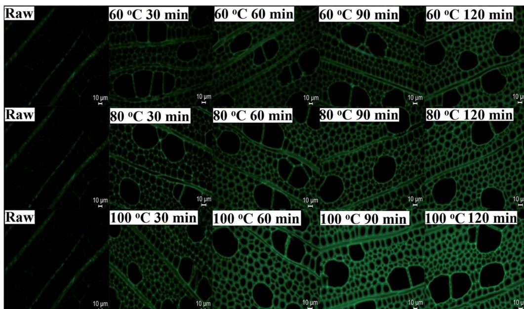
Fig. 1 Fluorescence microscope photos of poplar cell walls before (raw) and after dissolution treatments at different temperatures (60, 80, and 100 °C).
