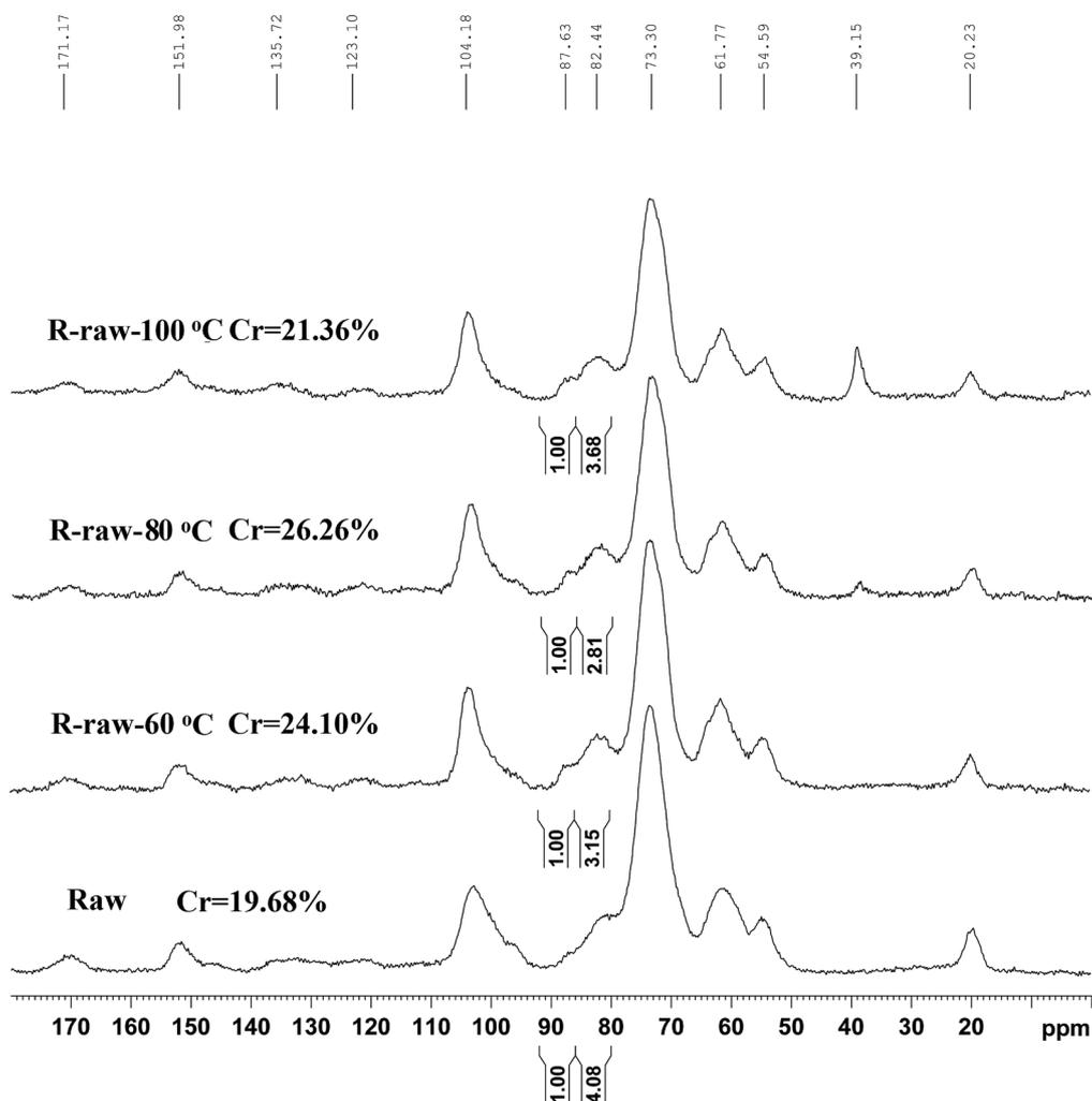
Fig. 3 CP/MAS <sup>13</sup>C-NMR spectra of the raw and regenerated ball-milled poplar wood.
