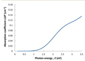
Fig. 12 Theoretical absorption spectrum of Cu<sub>0.5</sub>Co<sub>2.5</sub>O<sub>4</sub> clusters.
