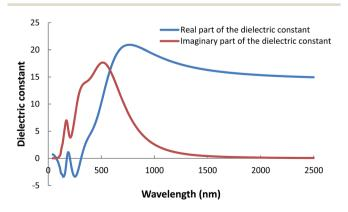
Fig. 13 Real and imaginary parts of dielectric constants of  $Cu_{0.5}Co_{2.5}O_4$  clusters.
