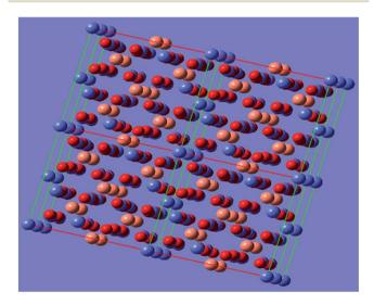
Fig. 1 Crystal structure of Cu-Co oxide coatings.
