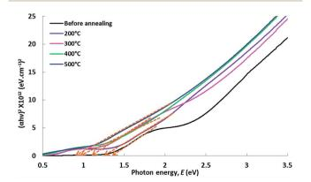
Fig. 3 Tauc plots of  $(\alpha h \nu)^2 vs$ . photon energy of Cu–Co oxide coatings before and after annealing.
