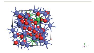
Fig. 10 Conventional unit cell of CuCo-oxide (Cu $_{0.5}$ Co $_{2.5}$ O $_{4}$ ) structure.
