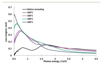
Fig. 8 Loss tangent vs. photon energy of Cu-Co oxide coatings before and after being annealed at different temperatures.
