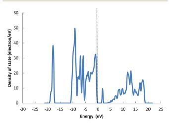
Fig. 11 Total density of states of CuCo-oxide (Cu<sub>0.5</sub>Co<sub>2.5</sub>O<sub>4</sub>) clusters.
