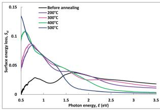
Fig. 9 Variation of volume energy loss and surface energy loss functions of Cu-Co oxide coatings before and after annealing
