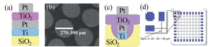
Fig. 1 (a) Schematic representation of a memristive cell; (b) SEM image of an array of Pt top dishes (270–300 μm in diameter) in a fabricated device; (c) schematic representation of a memristive unit in a crossbar array; (d) schematic representation of a crossbar array.
