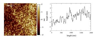
Fig. 2 AFM image of 1TPA, at  $2 \times 2 \mu m^2$ , (left) and surface profile (right).  $R_{\rm q}$  is 0.75  $\pm$  0.08 nm at this acquisition scale. False color vertical scale from -2 to 2 nm.
