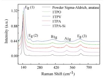
Fig. 5 Raman spectra acquired from  ${\rm TiO_2}$  thin films annealed in a variety of atmospheres together with the model Raman spectrum obtained from  ${\rm TiO_2}$  powder (Sigma Aldrich).
