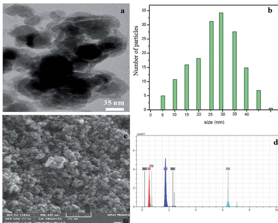
Fig. 3 TEM image of  $\text{Fe}_3\text{O}_4@SiO_2-MoO_3H$  (a), histogram of particle size distribution (b), SEM image of  $\text{Fe}_3\text{O}_4@SiO_2-MoO_3H$  (c) and EDAX spectrum of  $\text{Fe}_3\text{O}_4@SiO_2-MoO_3H$  (d).
