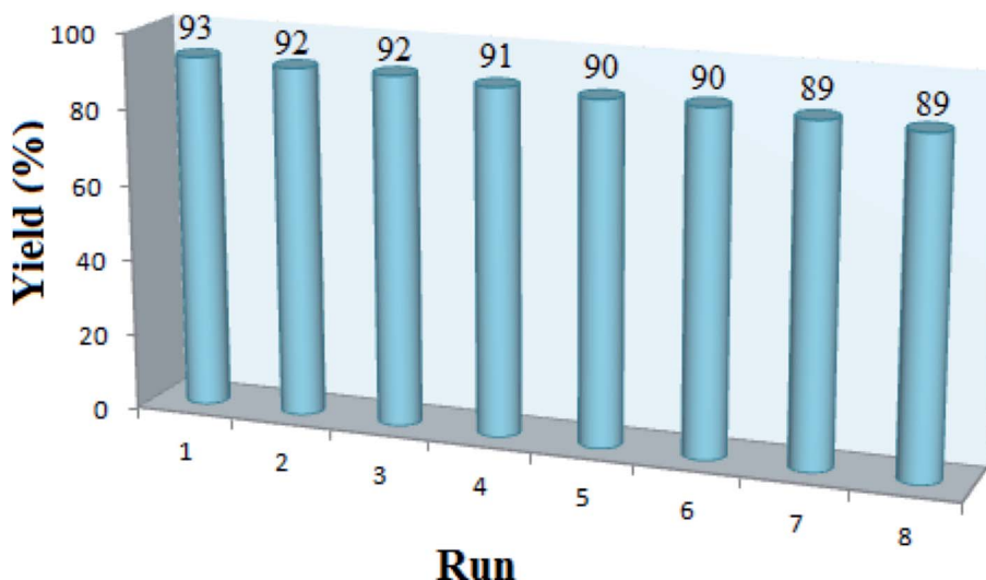
Fig. 8 Reusability of \text{Fe}_3\text{O}_4@\text{SiO}_2\text{-MoO}_3\text{H} for synthesis of 7a .
