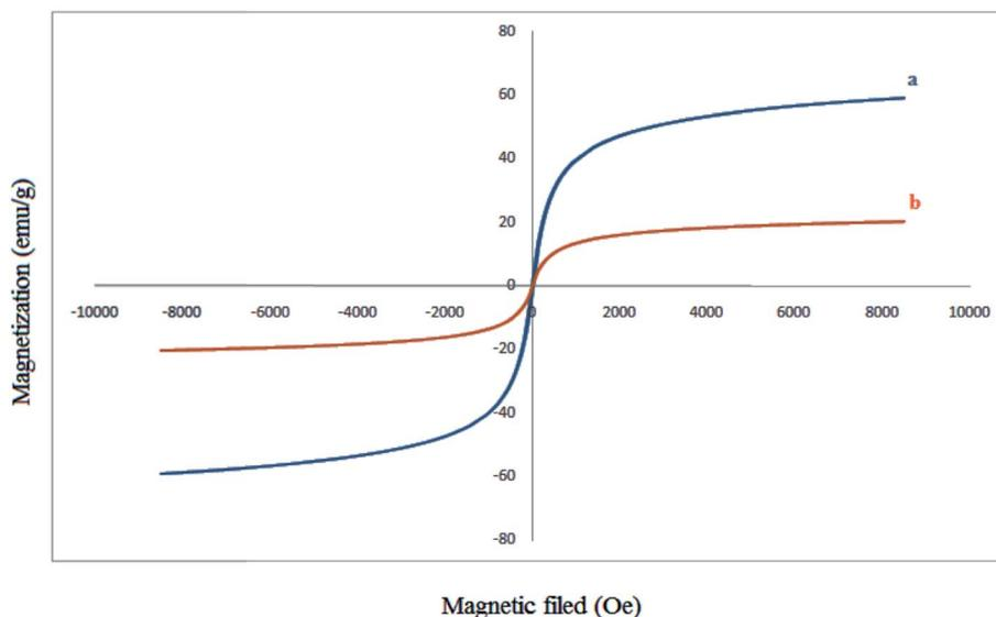
Fig. 5 Magnetization curves for the prepared  $\text{Fe}_3\text{O}_4$  MNPs (a) and  $\text{Fe}_3\text{O}_4@\text{SiO}_2\text{-MoO}_3\text{H}$  (b).
