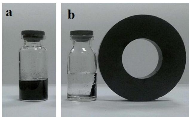
Fig. 6 Digital camera images of the aqueous solution with dispersed magnetic  $\text{Fe}_3\text{O}_4@SiO_2-MoO_3H$  composite particles (a) and after applied magnetic field (b).
