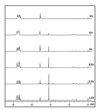
Fig. 3 <sup>1</sup>H NMR spectra at different time intervals during hydrolytic oxidation of phenylsilane.
