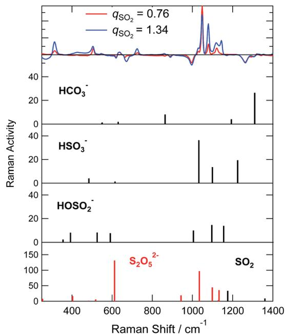
Fig. 8 Vibrational spectra of different anions calculated by DFT using aug-cc-pVTZ basis set and B3PW91 functional. The upper panel shows difference Raman spectra of  $[\text{P}_{4448}]\text{HCO}_3$  with different  $q_{\text{SO}_2}$  from neat  $[\text{P}_{4448}]\text{HCO}_3$ .
